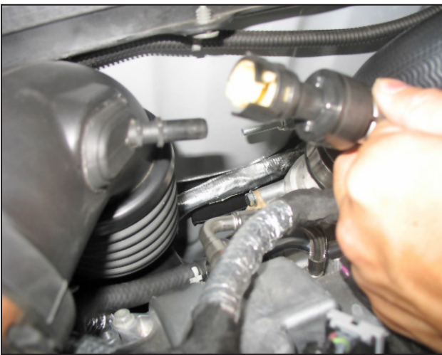
c. Disconnect the PCV line from the inlet tube by pressing the clip and pushing back.
