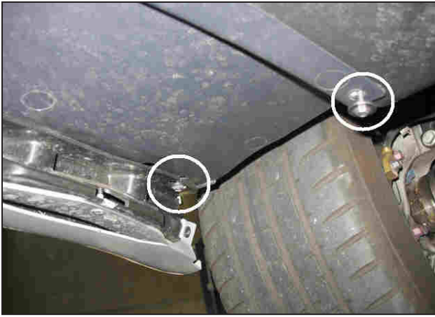
n. Remove the additional 7mm bolts and push clips on the corresponding bottom section.
