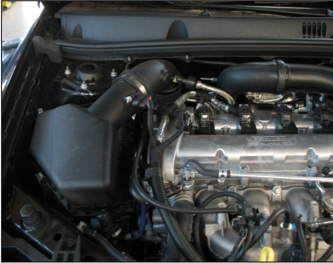
Stock air box system installed
