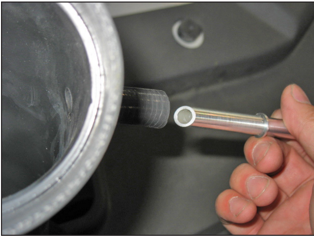
b. Insert the nipple breather (2-929) into the silicone adapter, with the orientation as indicated in the photo.
