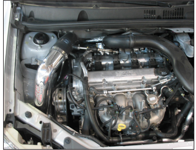
AEM® intake system installed
