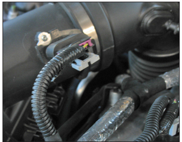
d. Remove the locking clip on the MAF sensor harness by pressing the clip with a small flathead screwdriver.
