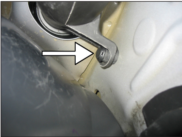
o. Locate the lower air induction pipe and remove the retaining clip on the top section with a flathead screwdriver.
