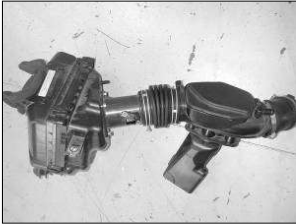
e. Pull directly upward on the air box to unplug it from the mounts. Remove the complete air box system from the vehicle.
