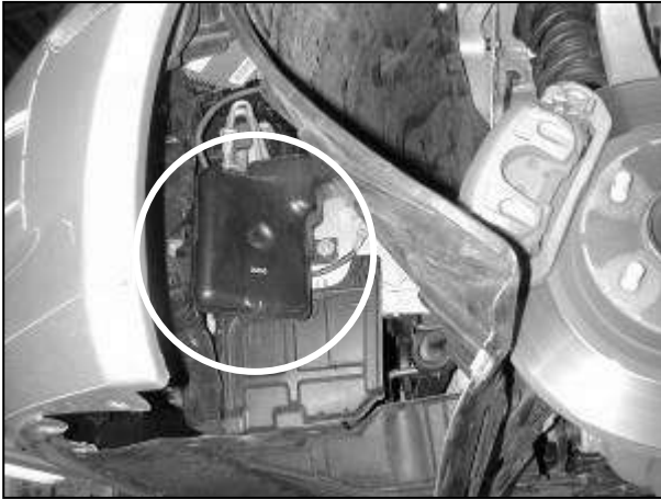
h. Peel back the splash guard and tuck it out of the way. Remove the lower resonant chamber circled in the picture.
