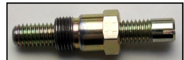
The large section screws into the sparking plug hole, and the center portion is adjusted to just stop the piston getting to TDC Adding a locknut to the top of the screw might be beneficial
