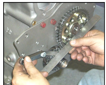
If these gears run out of line that's not good for chain life, or the gears!
