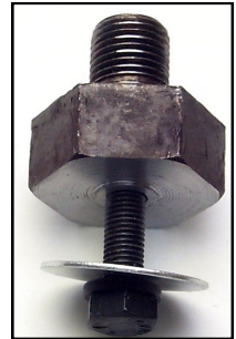
This crank bolt has a register on the front face to locate the degree wheel
