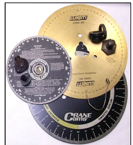
These are the degree wheels we use in the APT shop. The Lunati wheel has a separate lockable hub a Mini flywheel bolt holds it to the crank on BMC engines
