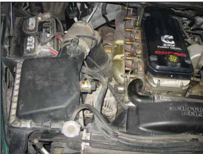
Factory air box system installed
