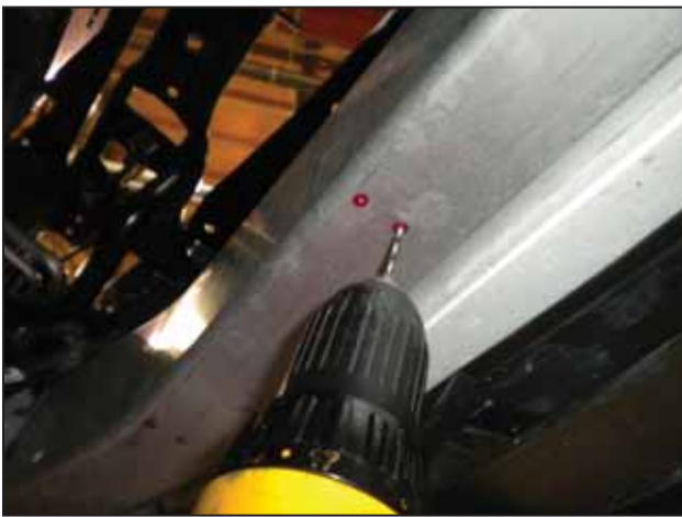
af. Use a 5/32 inch pilot drill for each of the 4 markings.
