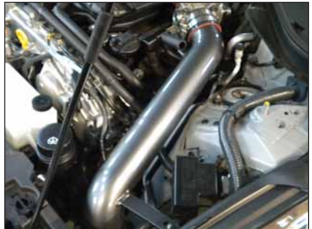
g. Install the driver side intake pipe 2-10011, aligning the upper bracket with the upper rubber mount and the lower bracket with the lower rubber mount.
