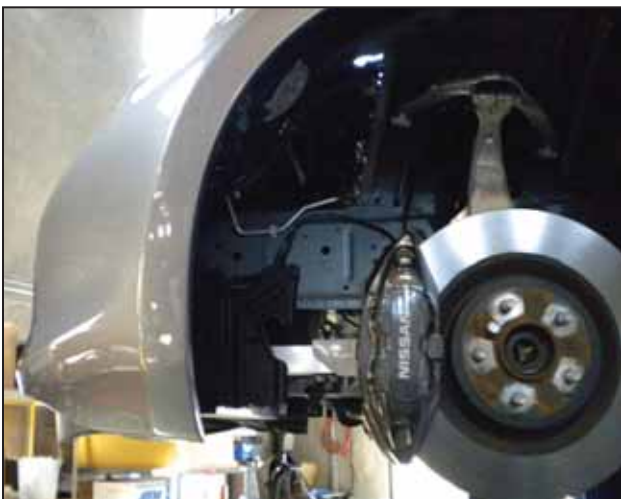
i. Remove the driver side fender liner.
