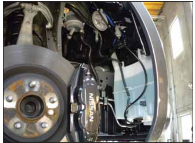
n. Remove the passenger side fender liner.
