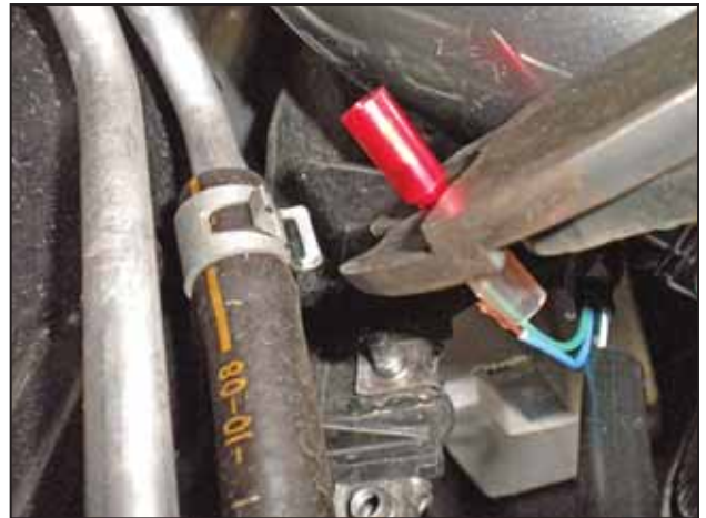
as. For 2009-2010 model year vehicles: Crimp the red female connector onto the green wire and the pink male connector onto the blue wire. For 2011 model year vehicles: Crimp the red female connector onto the red wire and the pink male connector onto the blue wire.
