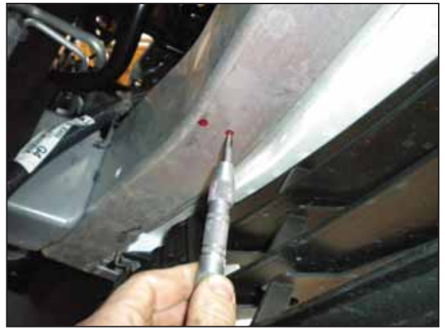
ae. Use a center punch to mark the holes.
