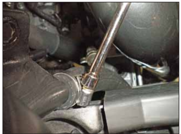
ao. Install the hose on the provided filler neck and tighten the clamp.
