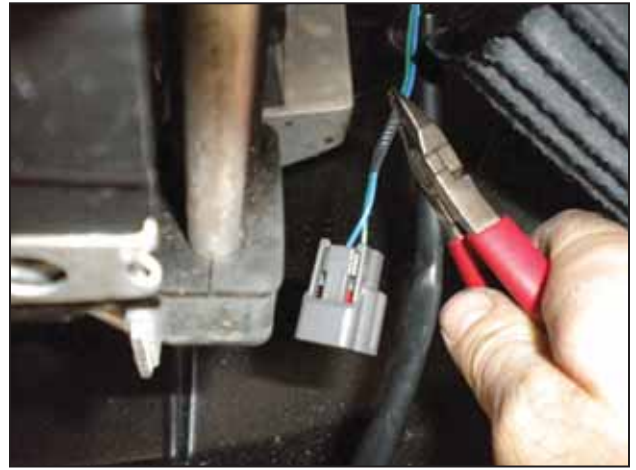
aq. Cut the stock pump connector off of the OEM harness leaving some wire on the connector. Do the same for the level sensor.
