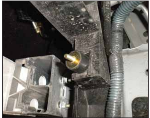
e. Remove the horn assembly. Thread the lower rubber mount where the horn bracket was previously installed.
