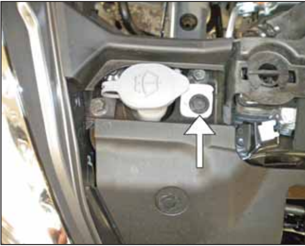
ao. Remove the clip next to the windshield washer filler cap as shown.
