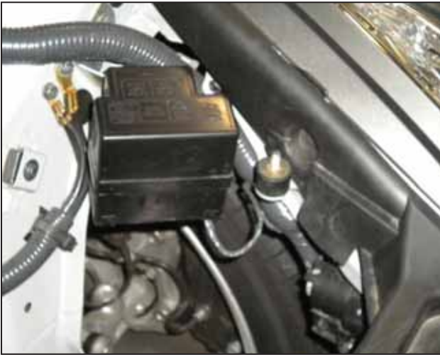
d. Thread the upper rubber mount in the driver side stock airbox mount location.
