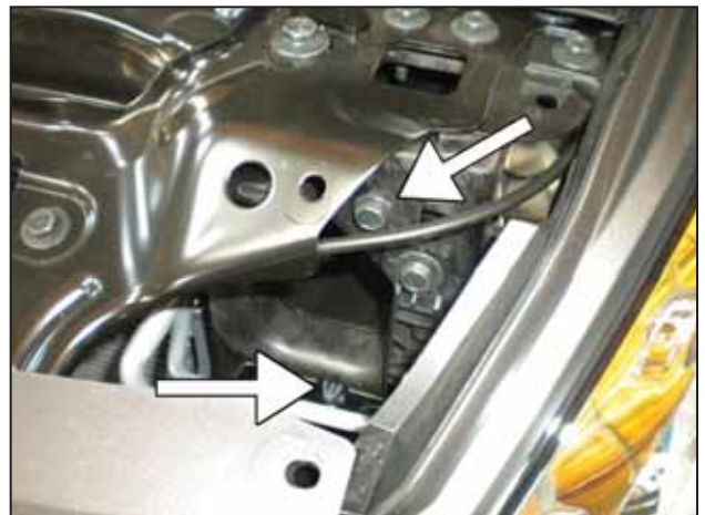
at. Remove the bolt and undo the clip to release the scoop on the driver side.
