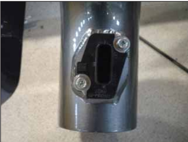
f. Install the mass air flow (MAF) sensor in the driver side intake pipe using the stock MAF bolts.
