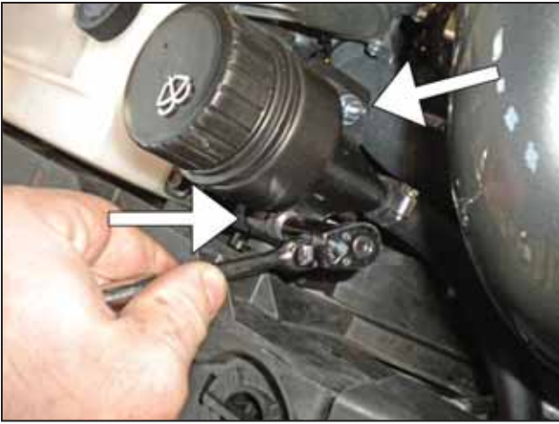
ap. Mount the filler neck to the bracket using two 6mm nuts and bolts.
