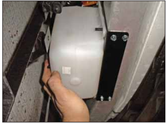
ak. Install the AEM® windshield washer bottle onto the installed bracket using the 4 supplied M6 washers and nuts.
