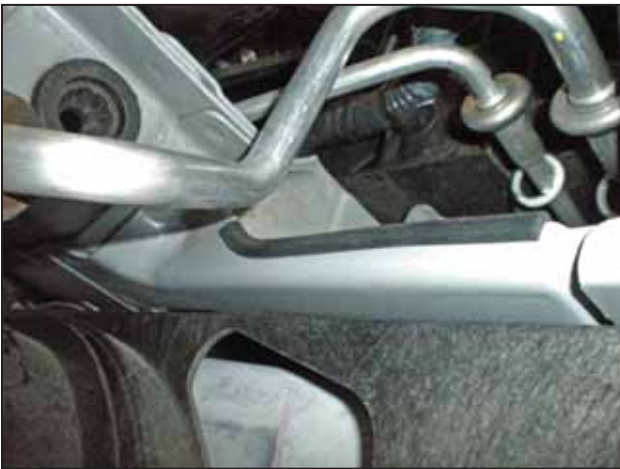
al. Install the rubber edge trim along the edge of the rail where the hose comes through the front core support.
