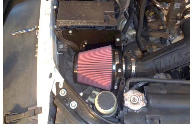
22. Install clamp (2) on air filter (1), install filter on filter adapter and tighten clamp.
