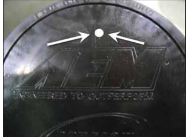
b. Drill 1/8" hole in lid of filter. Make sure no debris from the drilling operation gets inside the filter.
