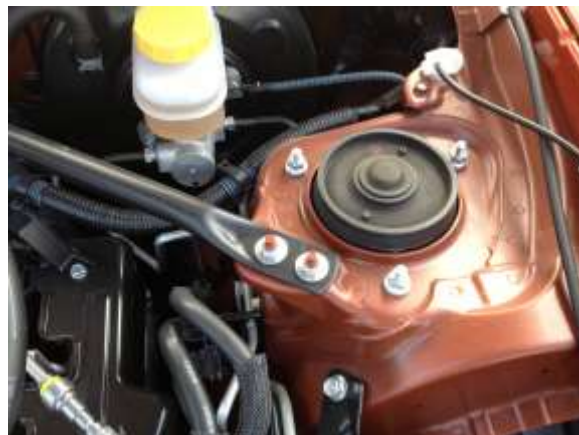
b. Loosen the fasteners securing the factory strut braces to the tower, and remove them. Loosen the 4 inner strut tower top nuts.
