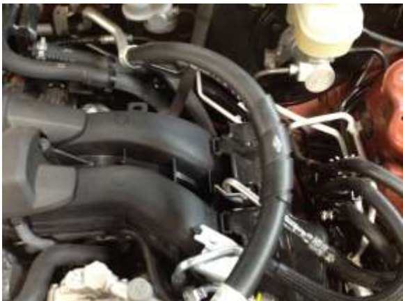
a. Install the included hose protector over the factory hose as shown.
