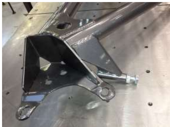
b. Assemble the included nut and bolt on the brake master cylinder brace.
