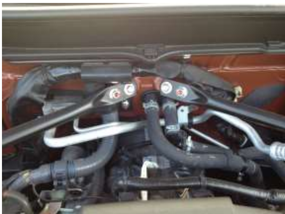
a. Loosen the fasteners securing the factory strut braces to the firewall.
