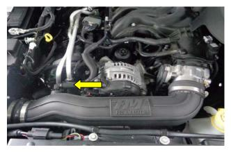
15. Install the FM intake tube assembly onto the airbox and the throttle body\*. Align and tighten all clamps for a satisfactory fit. Slip the crankcase vent hose onto the barbed fitting on the intake tube.
