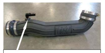
\*Do not exceed 8 ft/lbs torque; if necessary, apply Teflon thread tape to achieve proper clocking/torque.
