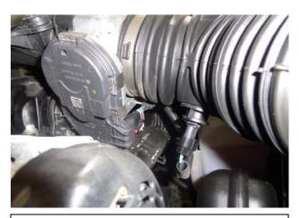
3. Disconnect the electrical plug from the air temperature sensor located on the underside of the intake tube near the throttle body by depressing the backside of the rocking tab and gently pulling away.
