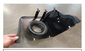
10. Install the rubber trim seal along the outer top and side edges as shown. Press fully into the groove starting from one end. Trim final length with metal shears for proper fitment.
