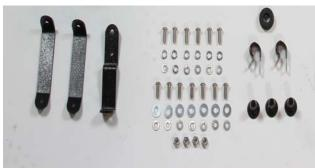
7. Begin assembly process of the FM cold air intake kit by removing all hardware and arranging by type and thread. This will facilitate an easier assembly process and lessen the chance of misplaced parts.
