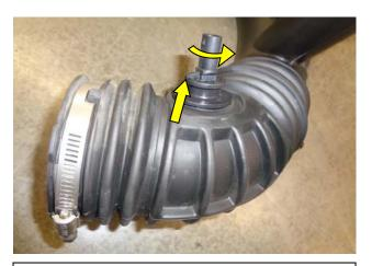
5. Remove the entire stock intake assembly from the vehicle by lifting straight up and out. Turn upsidedown on a flat surface and remove the air temp sensor from the intake tube by prying up the clocking tab with a flat screwdriver and rotating c-clockwise.
