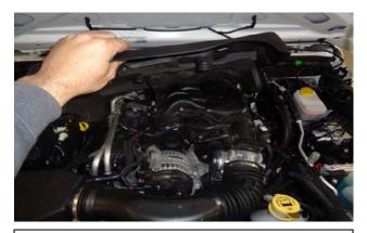
2. Remove the engine cover by grasping the front edge and lifting up, then pull forward. Unclip the coolant overflow hose from the air tube. We highly recommend that customers retain their factory air intake system.
