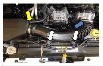
4. Loosen the hose clamp securing the factory intake tube to the throttle body. Remove the two bolts securing the stock intake tube/resonator to the front cross frame and retain. Disconnect the crank-case breather tube from the stock air-box.
