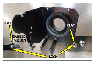
9. Install the metal brackets included in the kit using the supplied 1/4" screws/washers/nuts as shown. Then, install the barbed mounts onto the metal brackets using the 6mm screws/washers.
