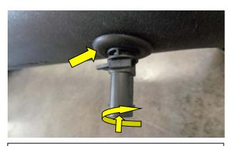
13. Insert the provided rubber grommet into the hole in the FM intake tube. Insert the pre-lubed stock air temperature sensor into the grommet by twisting clockwise and pressing inwards until seated as above.
