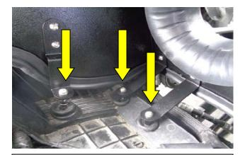
11. Install the heat shield assembly (minus the lid and FM intake tube) into the vehicle as shown above with the barbed mounts firmly pressed down until fully seated into the rubber grommets on the fender.
