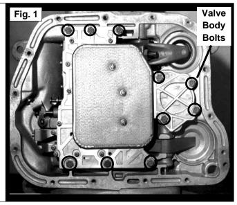
2. Remove and discard the filter. Carefully disassemble the valve body and lay out all the springs and valves as removed on a clean rag or paper towel (See Figure 2). Thoroughly clean each part (brake cleaner works well. Replace the stock limit valve spring with the supplied B&M limit valve spring (See Figure 2).
