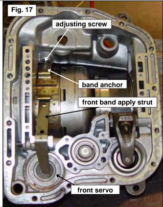
(1966 1969 23. thru transmissions only) Install the supplied B&M front servo inner return spring if not already equipped (later model transmissions do not require any front servo modification) (See Figure 18). The later model front servo piston has a larger (over 1/2") diameter center pin and does not require disassembly any or modification.
