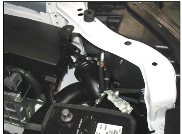
l. Remove the push-in clip from the air horn inlet. Remove the inlet from the remainder of the tubing located in the fender well.
