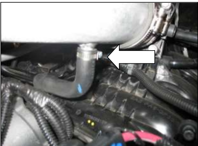
n. Attach the breather hose to the inlet pipe and secure with 1" hose clamp.
