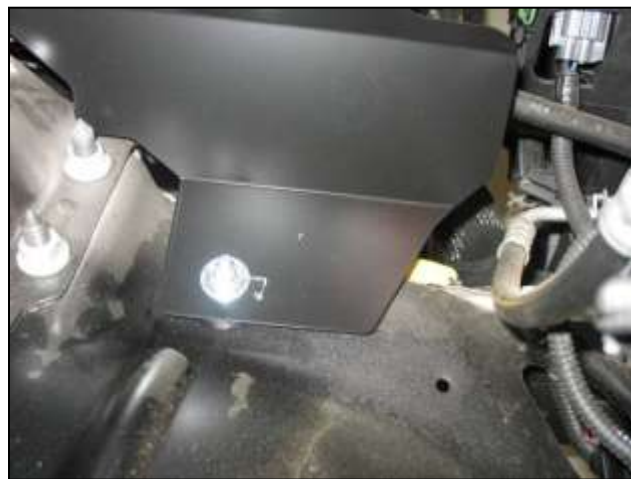
g. Secure the bottom of the heat shield with the fender washer (559999) and nylok nut (1-2074).
