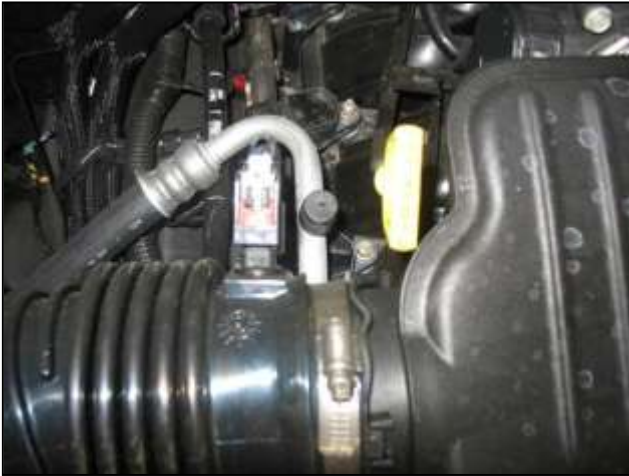
a. Disconnect the Inlet Air Temperature (IAT) sensor connector. Push up the on the release (red) and depress the connector (black).
