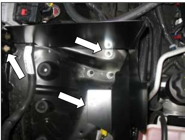
i. Check clearance around the body and the heat shield. Tighten all mounting points.
