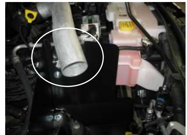
o. Ensure there is sufficient clearance around the inlet pipe and the heat shield.
