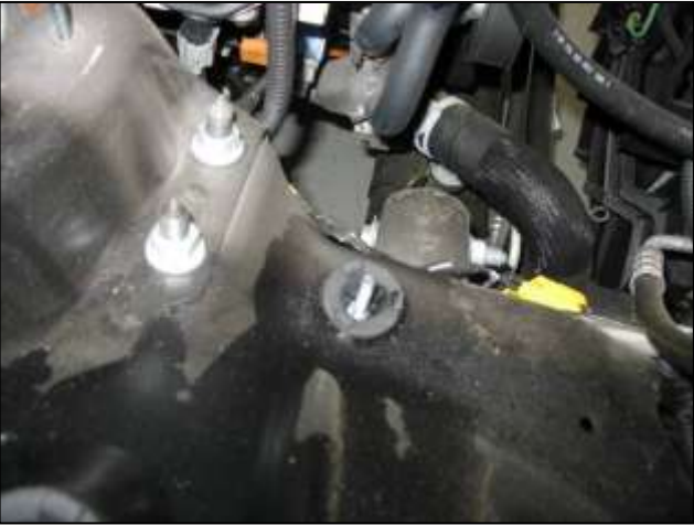
b. Insert the 1/4-20 bolt (1-2072) and 1/4 washer (1-3028) from underneath the grommet through the fender well.
