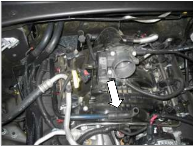
f. The breather hose should be positioned as shown. The hose outlet should sit vertical.
