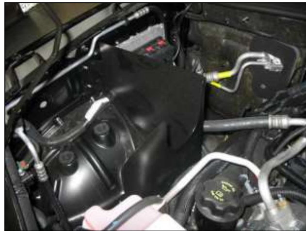
e. Insert the heat shield as shown. Align the heat shield to the studs in previous step. The bottom of the heat shield should align with the stud from step 3(c).
