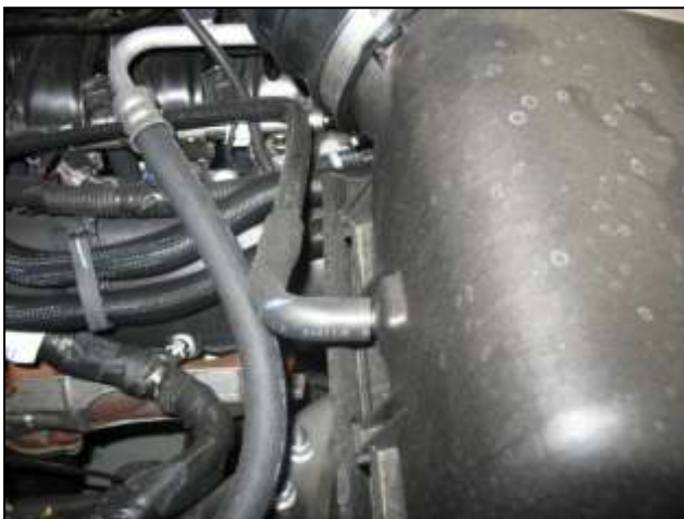
c. Remove the PCV breather tube from the air box. Remove the air box and inlet tube.
