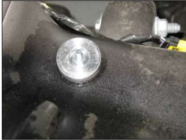
c. Install the aluminum stand (2-670) over the bolt installed in the previous step. Secure the assembly with the 1/4-20 nut (1-2073) and tighten.
