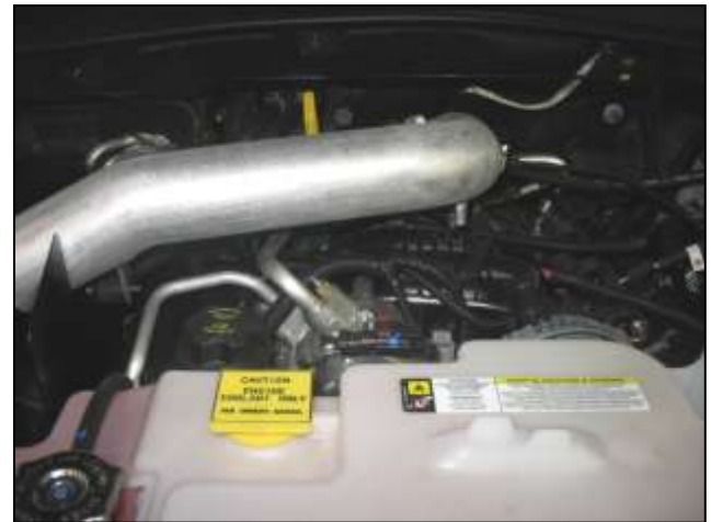
m. Insert the inlet pipe into the reducer coupler. Align the bracket with the rubber mount on the heat shield. Install the IAT into the rubber grommet and reconnect the wire harness.
