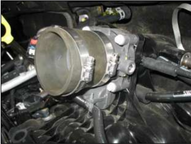
j. Attach the reducer coupler to the throttle body and secure with #44 and #48 hose clamps.
