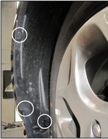
i. Remove the 2 T25 screws and 1 plastic clip from the front driver and passenger wheel wells as shown. You may need to turn the wheels to access T25 screws.
