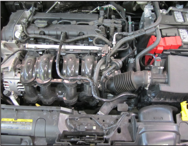
a. Stock air box system installed.
