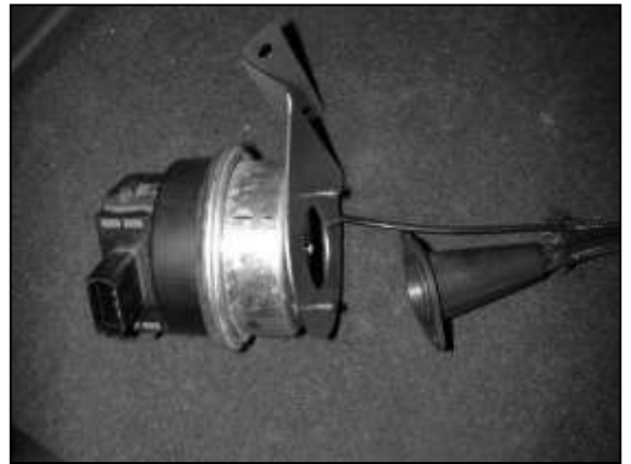
h. Insert the mounting studs of the cruise control unit into the AEM ® bracket as shown.
