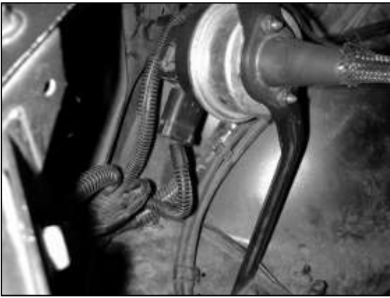
c. Unplug the electrical connection from the cruise control unit by pulling the red tab out, then pulling off the connector.
