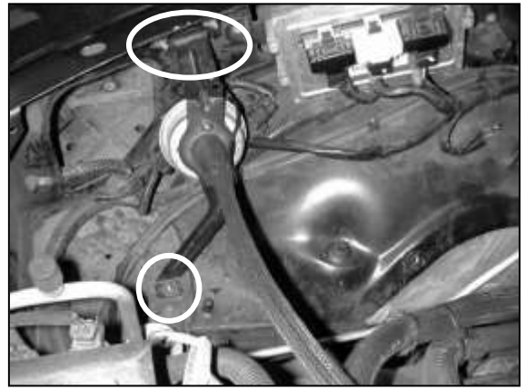
d. Remove the three nuts from the cruise control mounting bracket and remove the unit from the engine bay.
