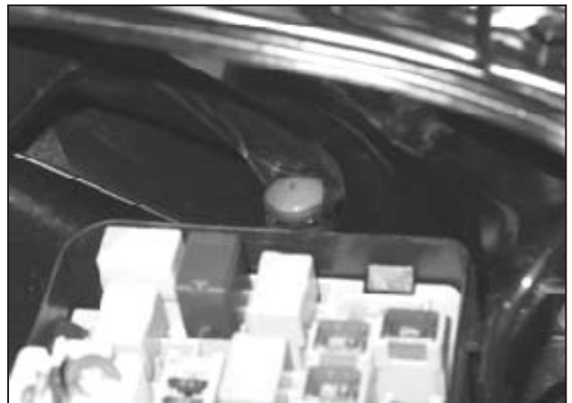
n. Remove the second clip from the lower intake tube. Then remove the lower intake tube.
