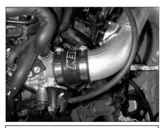
j. Loosely install the 2.75" silicone hose on to the  $\mathsf{AEM}^{\otimes}$  intake pipe with the two #44 hose clamps. Insert the AEM intake pipe into the engine bay, filter end first. The pipe should pass under the bundle of wires going to the fuse box. Loosely secure the silicone hose to the throttle body.
