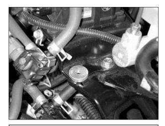
c. Place the supplied VSV bracket spacer in line with the hole exposed in the previous step.
