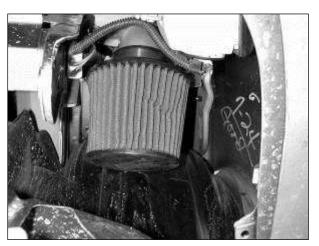
p. Install the AEM® air filter on the end of the AEM® intake pipe. Ensure the air filter does not contact any part of the vehicle and tighten the #48 hose clamp.
