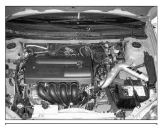
AEM® intake system installed
