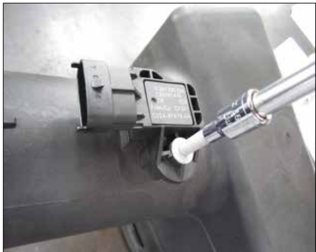
i. Remove the Intake air temp sensor using a 4mm socket to remove the stud holding the sensor. For vehicles using a MAF sensor move on to step J.
