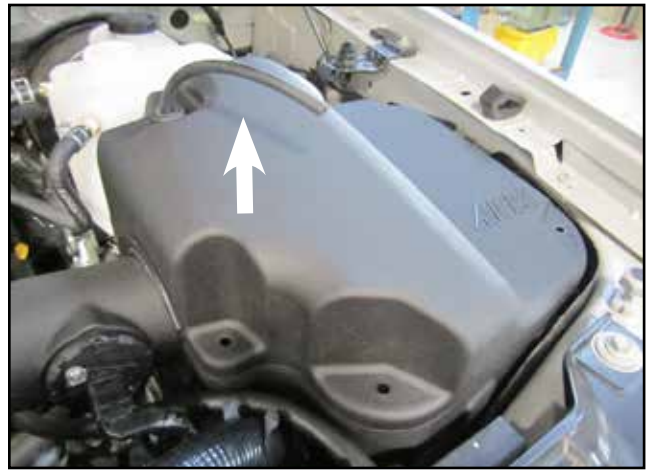
cc. Feed the filter minder hose (T) up through the grommet in the upper air box and place it on top of the lower air box.
