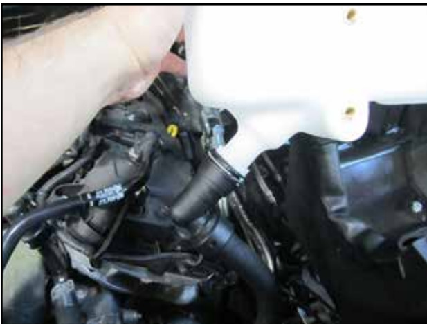
l. Connect the lower coolant hose by pressing it in place until it clicks in.
