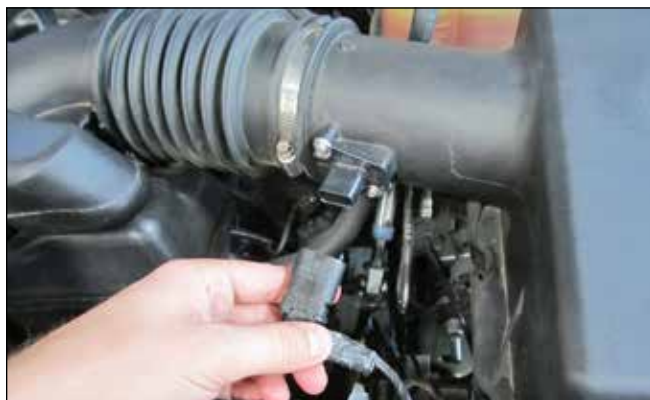
d. On vehicles equipped with a mass air sensor, release the red locking tab and then disconnect the mass air sensor electrical connection. On vehicles equipped with a tempature sensor, disconnect the electrical connection and then unhook the wiring harness from the stud.
