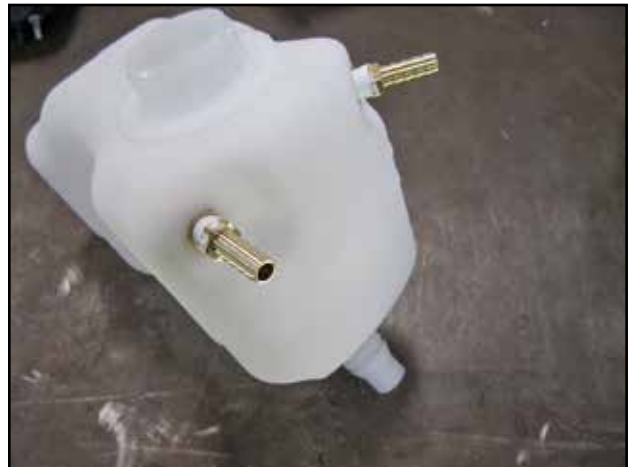
k. Install two brass barbs (S) into the AEM coolant reservoir (U) using thread sealant to seal the threads.
