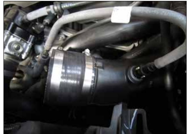
w. Install coupler (R) and the two hose clamps (AB) onto the driver's side turbo inlet tube.
