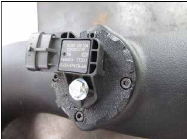
v. For Trucks using a IAT sensor install the OEM sensor with the supplied M6 Bolt (AD).
