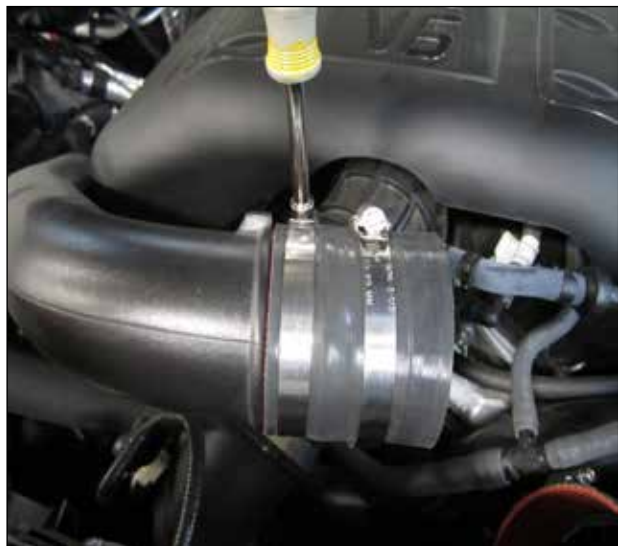
x. Install coupler (Q) and the two hose clamps (Z) onto the passenger side turbo inlet tube.
