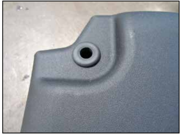
aa. Install the filter minder grommet (E) in the AEM air box lid (W).
