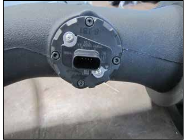
u. For Trucks using a MAF sensor Install the OEM sensor with the supplied M4 bolts (J). Trucks using an intake Air Temp Sensor move to step v.
