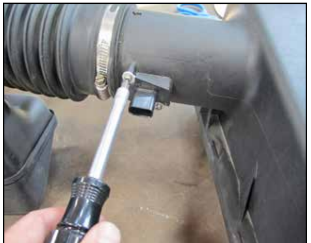
j. Remove the MAF sensor and set it aside for future use.
