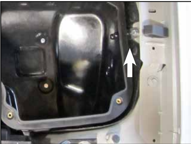
j. Secure the AEM lower air box bracket (H) to the fender support with the provided M8 bolt (K).
