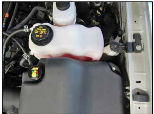
ee. Refill the coolant drained in step 2m and check for leaks, then secure the cap.
