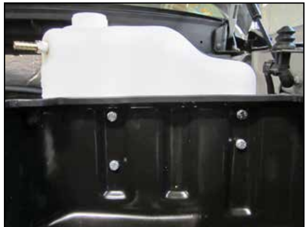
m. Install the AEM reservoir (U) and secure it to the AEM lower air box using the four M6 bolts (N) and washers (M) provided.
