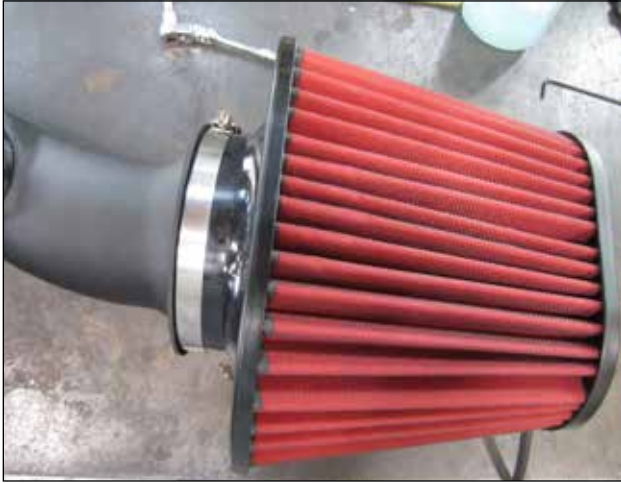
t. Install the filter (R) and #80 clamp (O) onto the filter grommet as shown.
