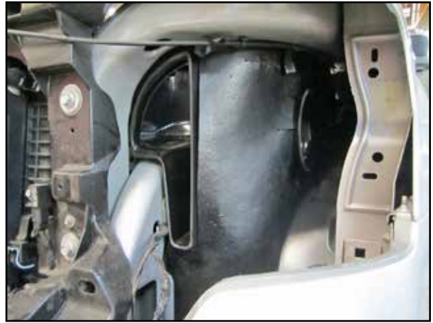
i. Make sure that the side inlet scoop is protruding through the inner fender liner as shown.
