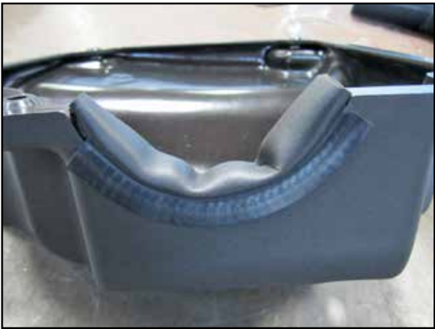
bb. Install the bulb seal (X) and (Y) around the U-shaped opening on the AEM air box.
