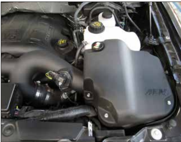
dd. Plug the filter minder hose onto the filter minder(F) and press it into the grommet on the upper air box. Secure the upper air box with the five supplied M6 bolts(G).
