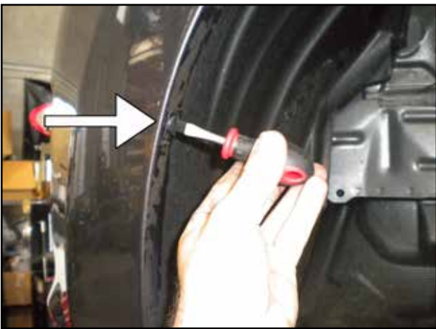
n. Remove the 5 clips securing the driver side fender liner.
