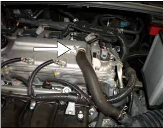
a. Remove the hose from the valve cover inlet.
