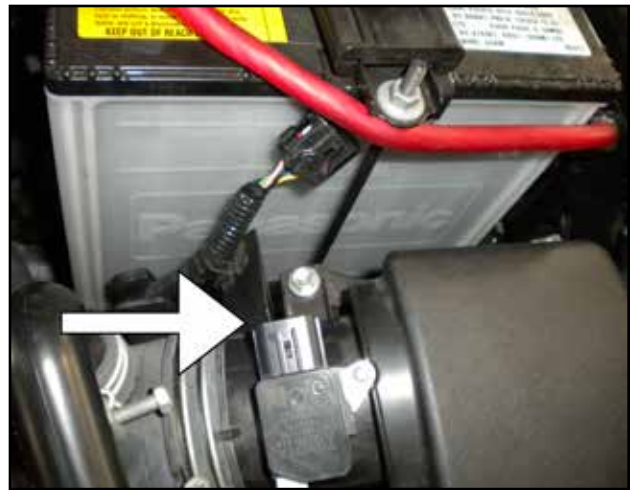
b. Unplug the MAF sensor wire harness from the MAF sensor.
