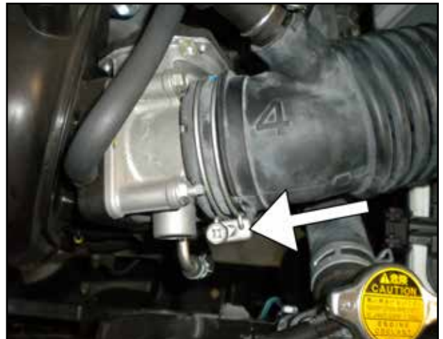
d. Loosen the hose clamp securing the inlet tube to the throttle body.
