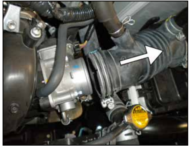
f. Remove the inlet hose from the throttle body.
