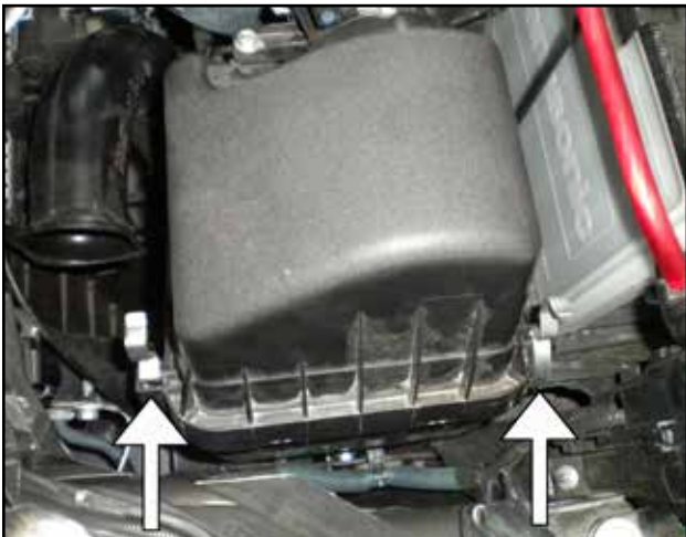
c. Release the 2 clips that secure the airbox lid.
