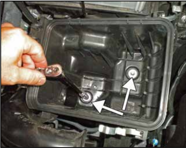
k. Remove the two 10mm bolts securing the lower airbox assembly.
