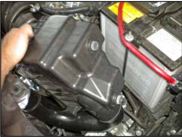
m. Remove the lower airbox assembly from the vehicle.
