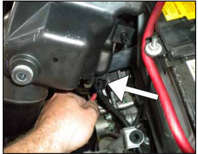
l. Rotate the lower airbox assembly and unclip the MAF sensor wire harness from the airbox.
