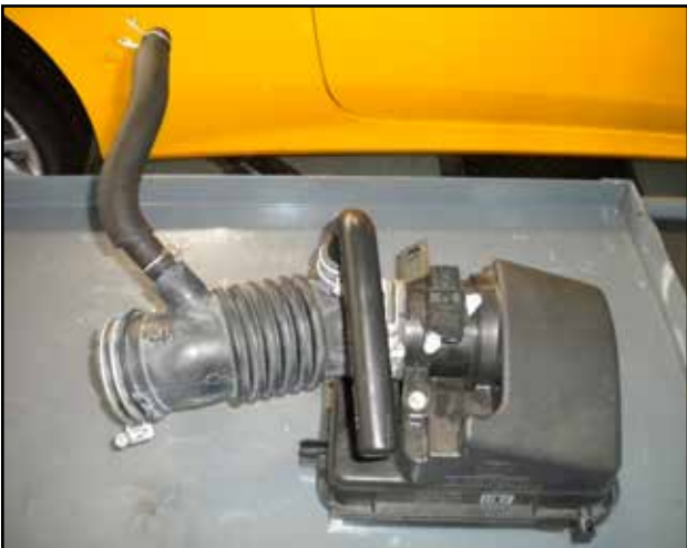
i. Remove the upper airbox assembly from the vehicle.
