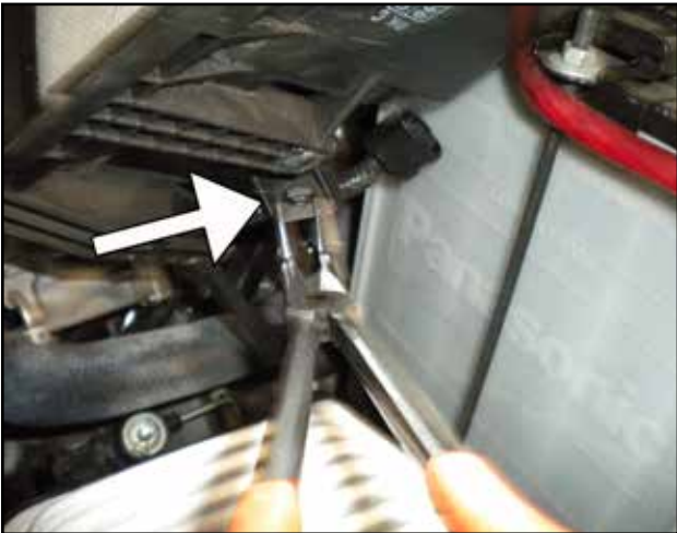
g. Lift the airbox lid to access and remove the clip securing the MAF sensor wire harness.
