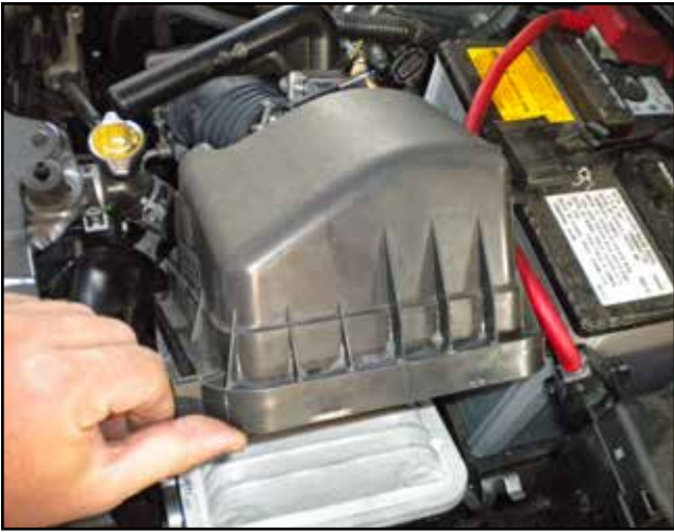
e. Lift the airbox lid from the lower portion of the airbox system.
