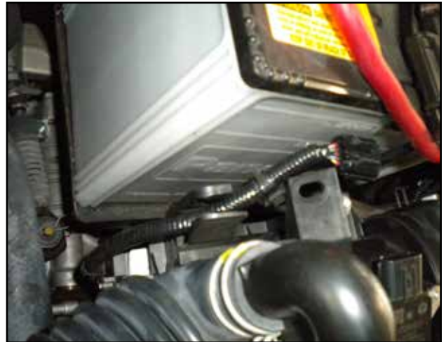
h. Remove the MAF sensor wire harness from the airbox lid.
