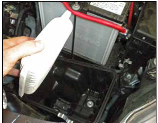
j. Remove air filter element from the lower airbox assembly.
