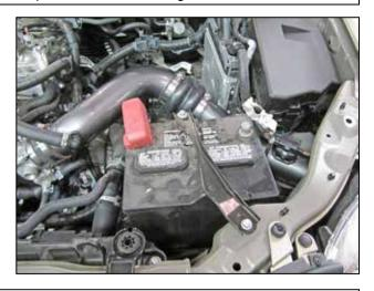
m. Install the plastic battery tray, the battery and the battery tie down. Reconnect the positive battery terminal. Refer to the owner's manual for specific details regarding battery installation.
