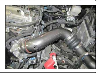
i. Install the upper inlet pipe ensuring it is evenly distributed in the coupler and hump hose. Secure the pipe in place by tightening the hose clamps.
