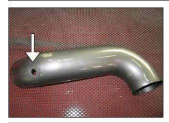
h. Install the grommet into the hole of the upper inlet pipe.
