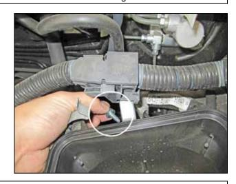
j. Remove the bolt that secures the harness bracket to the back of the lower air filter housing.
