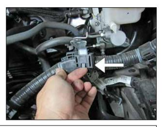
I. Remove the metal bracket from the harness, lift the tab up and remove the bracket as shown.
