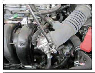
g. Loosen the hose clamp that secures the intake hose to the throttle body.
