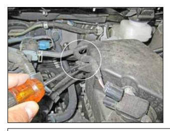
e. Remove the MAF sensor harness clip from the air filter housing.
