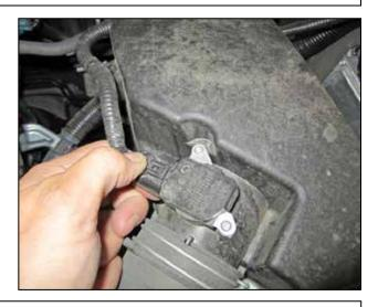
d. Unplug the MAF harness connector from the MAF sensor.
