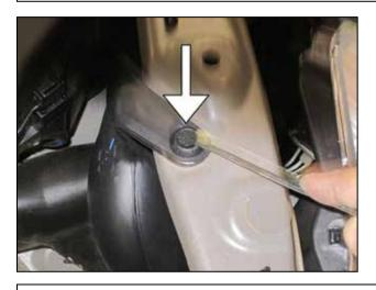
m. Behind the headlights locate the clip securing the intake duct. Remove the clip and then remove the duct.
