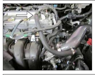
I. Attach the other end of the hose onto the PCV vent and secured it with a supplied hose clamp (# 99024.032).
