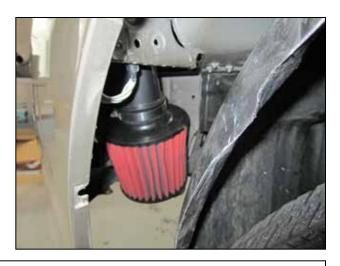
e. Attach the air filter to the lower end of the lower inlet pipe with hose clamp #9444.
