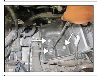
i. Remove the 3 bolts that secure the lower air filter housing to the vehicle chassis.
