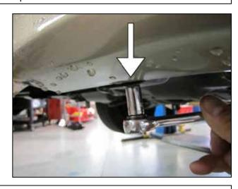
n. Locate the 2 bolts at the bottom of the vehicle that secure the lower portion of the plastic wheel well liner to the front bumper; remove these two bolts.
