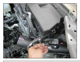
d. Route the MAF sensor harness to the ETI module as shown, connect the harness connector to the ETI module.
