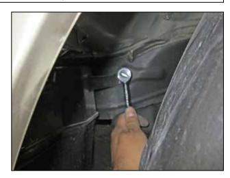
p. Remove the 2 bolts and nut that secure the resonator box to the inner fender well, remove the resonator box from the vehicle.
