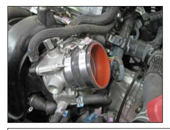
f. Attach the throttle body coupler to the throttle body with a #9444 and #9440 hose clamp.
