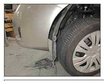
o. Remove the clips securing the wheel well liner to the inner fender allowing it to hang down as shown.
