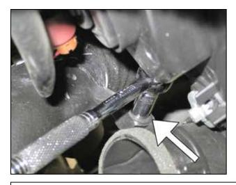
q. Locate the air duct and hose assembly behind the driver side headlight. Remove the bolt that secures the hose in its folded position.
