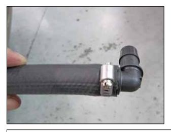
j. Slide the 5/8" hose over the  $90^{\circ}$  plastic elbow and secure it with the hose clamp (# 99024.032).
