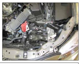
b. Disconnect the positive battery terminal. Remove the battery and plastic battery tray. Refer to the owner's manual for specific details regarding battery removal.
