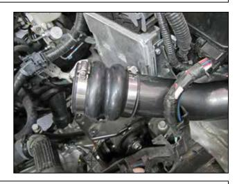
g. Slip the double hump hose onto the inlet pipe, but do not completely tighten the #9444 hose clamps.
