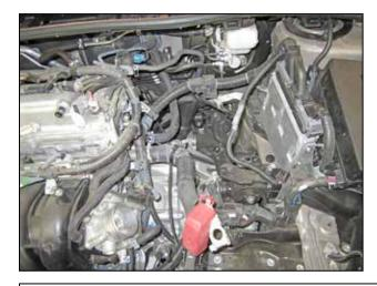
k. Remove the lower air filter housing.
