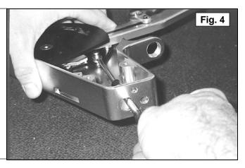
5. Push the cable anchor tab flush to the rear of the shifter body. Align the 17/64" cable flange hole with the 9/32" hole in the shifter body. Be sure to use the hole directly above the large cable access hole. Install the 1/4" bolt from the outside of the shifter body through the cable mounting flange until the bolt sticks through to the inside of the shifter body. Place the supplied 1/4" washer over the exposed threads on the inside, then thread on the 1/4" nut and tighten (See Figure 5).
