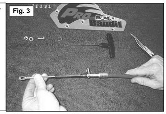
4. Insert the extended stamped loop end of the cable through the largest access hole in the rear of the shifter body. Slip the stamped loop cable end over the cable attachment pin at the rear of the shifter stick and attach the supplied e-clip to the pin. Check to make sure you have the e-clip firmly and accurately in the locating groove in the pin (See Figure 4).
