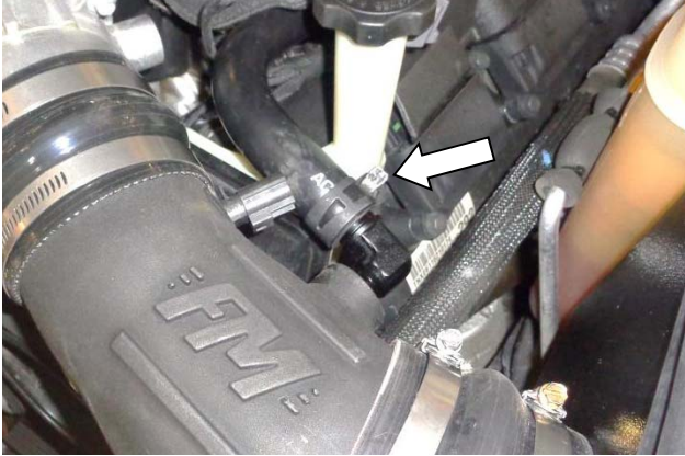
18. Secure PCV hose to barbed elbow with pinch clamp (19).
