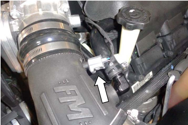
19. Reinstall the connector on the inlet temperature sensor and verify that the connector is secure.
