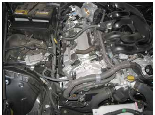
n. Factory airbox system removed.
