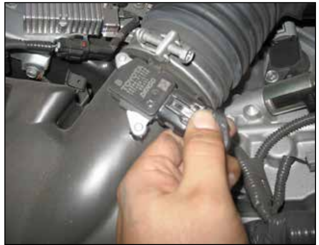
h. Disconnect the MAF harness from the MAF sensor.
