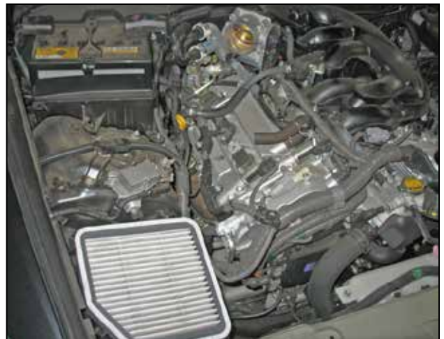
j. Unclip the 4 clips securing the airbox lid to the airbox. Remove the inlet tube/airbox lid assembly from the vehicle.
