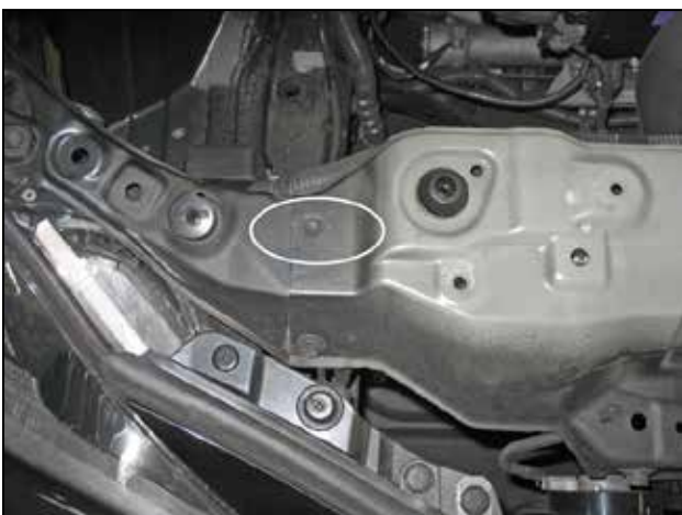
o. Remove the stock bolt shown, this will bolt will be reused during the installation of the AEM® intake system.
