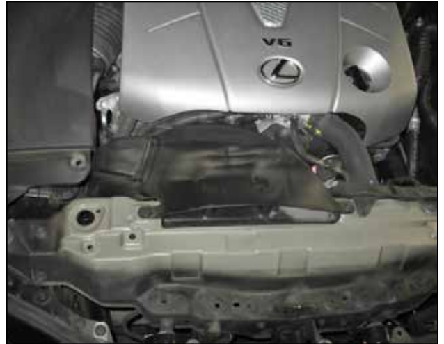
b. Remove the 11 push-in clips.
