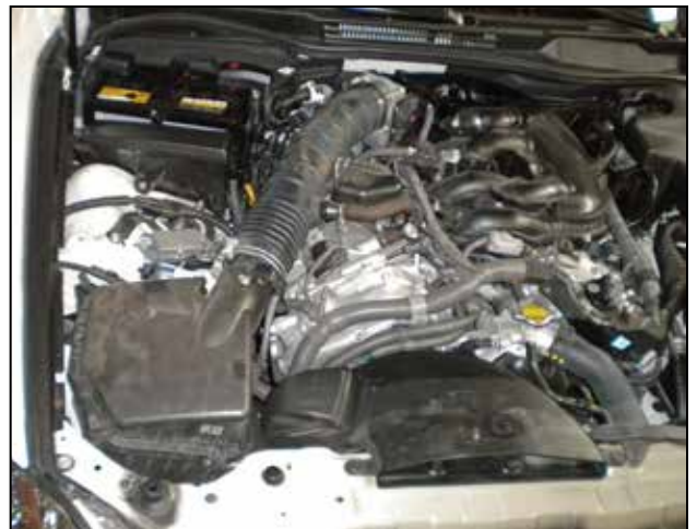
d. Remove the engine cover.
