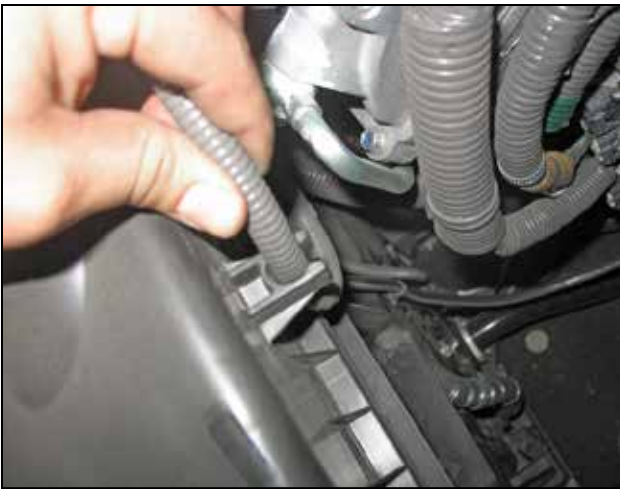
g. Disconnect the MAF harness from the lower airbox.
