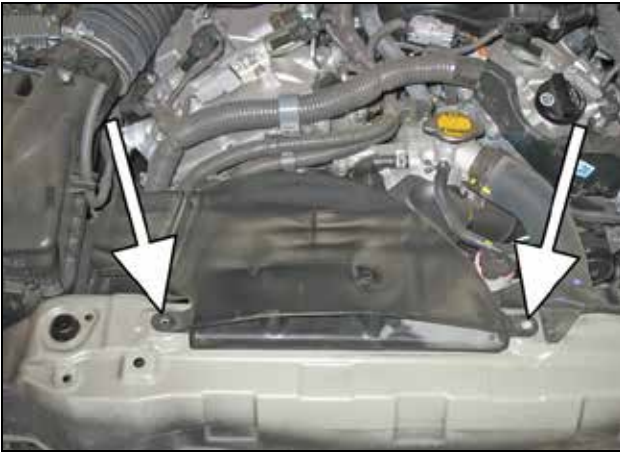
e. Remove the bolt and clip securing the inlet duct, then remove the inlet duct.
