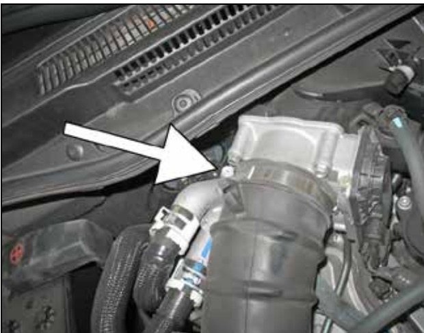
i. Loosen the hose clamp securing the inlet tube to the throttle body.
