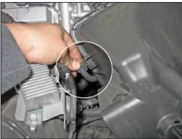
m. Flip the lower airbox and disconnect the zip tie from the lower airbox bracket.
