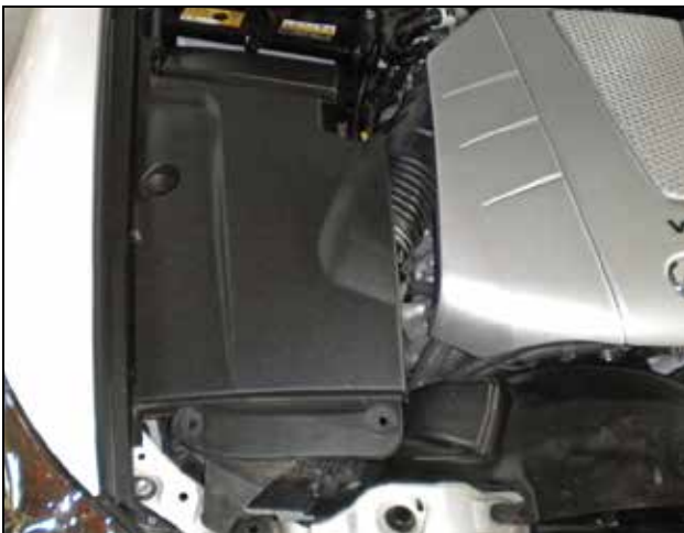
c. Remove the engine bay side cover.
