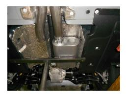
6) Place a supplied 3" clamp onto the inlet neck of both mufflers. Slide the mufflers onto the back of the Scavenger pipe assembly and support with stands. Level the mufflers and tighten the clamps enough to hold, but still allow for adjustment.
