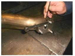
2) Then mount with the spacers and washers attached. Tighten securely.
