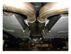
5) Begin the installation by placing a supplied 2-3/4" clamp onto each of the inlets of the Scavenger pipe #26522S. Then place the Scavenger pipe onto the back of the stock head pipes (the offset outlet pipe should be oriented to the right side). Level and center the assembly in the drive line tunnel and support with a stand. Tighten the two clamps enough to hold, but still allow for adjustment.
