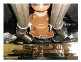
2) Place a stand under the center resonator just forward of the axle-back muffler assemblies. Loosen the clamps at the inlets of the Flowmaster or Hurst axle-back mufflers.
