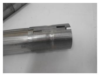
1) Slide a supplied **TB810S** adapter pipe onto the end of each outlet of the **86320S** Y-pipe assembly. Place a supplied clamp onto the connections and tighten enough to hold.
