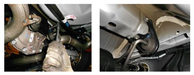
3) Using a 13mm wrench, loosen the two hangers just behind the rear differential from the cross member and the two hanger mounts at the rear of the vehicle from the frame. Slide the muffler assemblies toward the rear of the vehicle to disengage them from the factory system. Leave them hanging in place for re-assembly onto the Flowmaster Y-pipe assembly.
