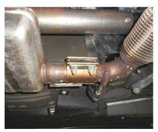
3) Using a 15mm wrench, loosen the two nuts at the clamp connection in the center of the vehicle. Use a small screwdriver to lift the clip and with the help of an assistant, carefully lower the stands at the rear of the resonator and slide the system toward the rear and off of the front pipe. Lower the resonator from the vehicle. The clamp should remain on the factory front pipe as it will be re-used with the new Flowmaster system.
