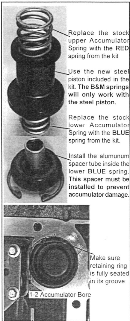
Figure 6. 1-2 Accumulator assembly
