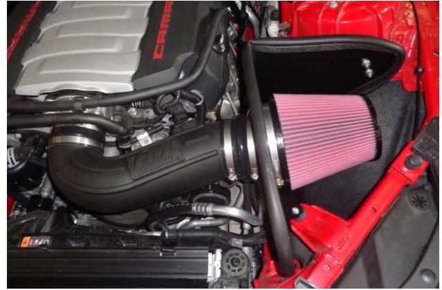
27. Install clamp (2) on air filter (1), install filter on filter adapter and tighten clamp.
