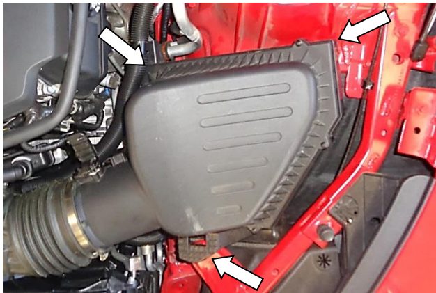
7. Grasp each corner of the airbox – one at a time – and firmly pull straight off to release each mount pin from its rubber grommet. After releasing all three pins, remove the airbox and intake tube.
