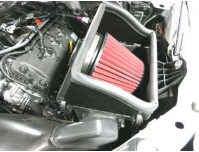
e. Place heat shield into factory lower air box. Do not secure clips until intake tube is in place.
