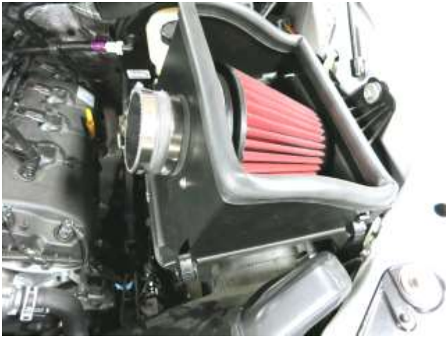
f. Install included straight hose coupler onto filter adapter and secure with provided hose clamp.
