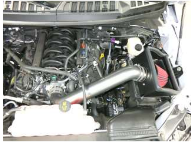
p. Finished installation of AEM Intake System.
