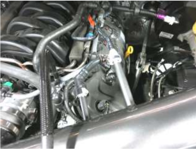
i. Connect factory EVAP and crank case vent connections to fittings on intake tube.
