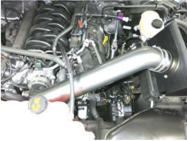
h. Install intake tube at throttle body first, then at air filter. Adjust tube position in couplers for best fit, then secure by tightening hose clamps. Secure heat shield using factory clips at this time.
