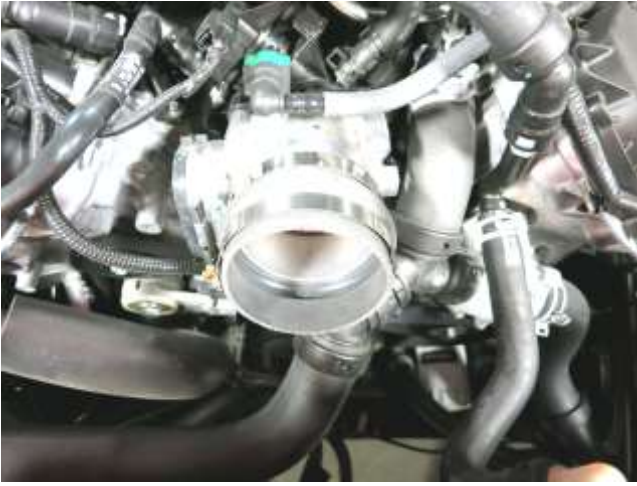
g. Install hump hose coupler onto throttle body and secure with provided hose clamp.
