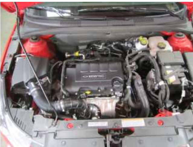
STOCK INTAKE INSTALLED
