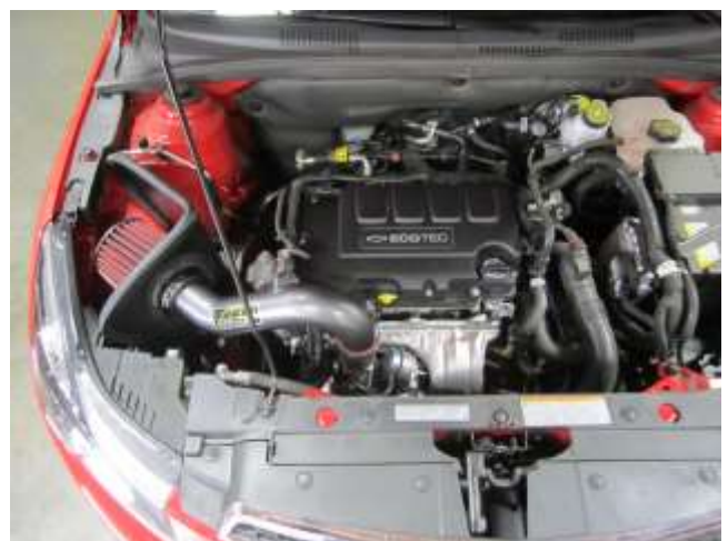
AEM INTAKE INSTALLED
