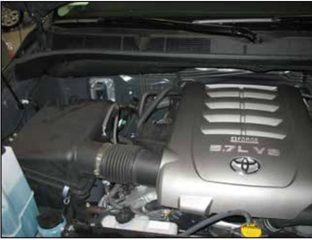
Factory airbox system installed
