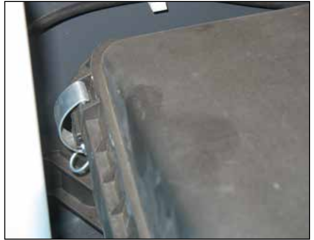
f. Unclip the second airbox clip.
