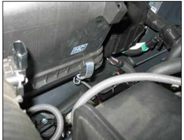
h. Unclip the forth airbox clip.
