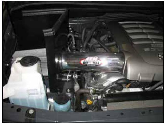
AEM® intake system installed
