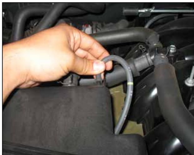
b. Remove the small hose located on the back of the inlet resonator.
