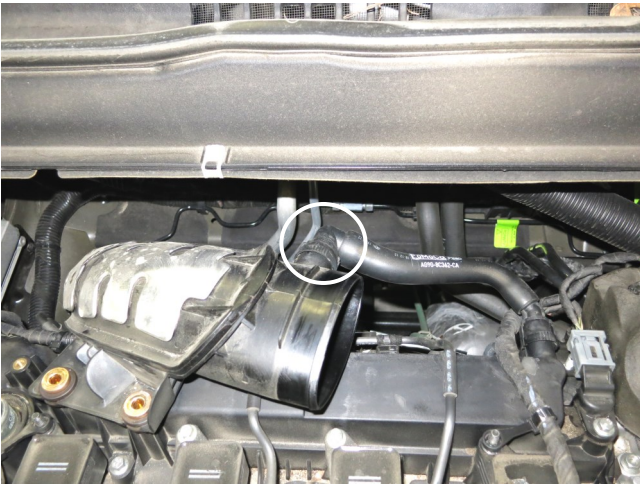
g. Squeeze the connector and slide the connector off of the intake tube.
