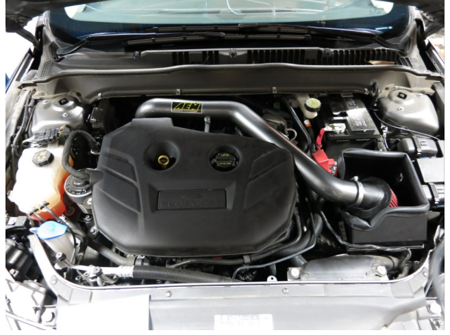
AEM INTAKE INSTALLED
