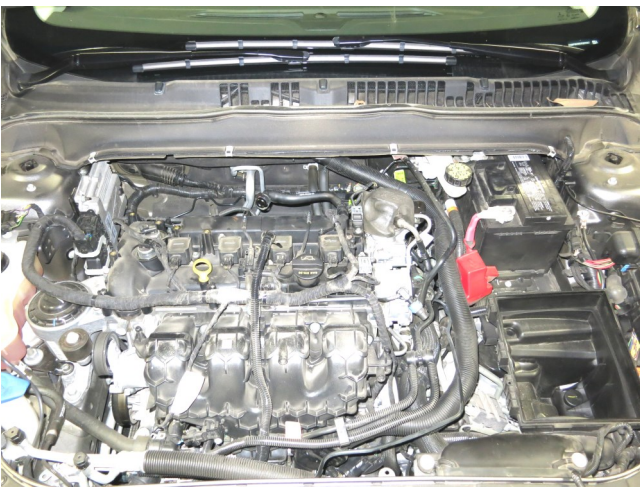
i. Remove the upper intake tube. Your engine bay should now look like this.
