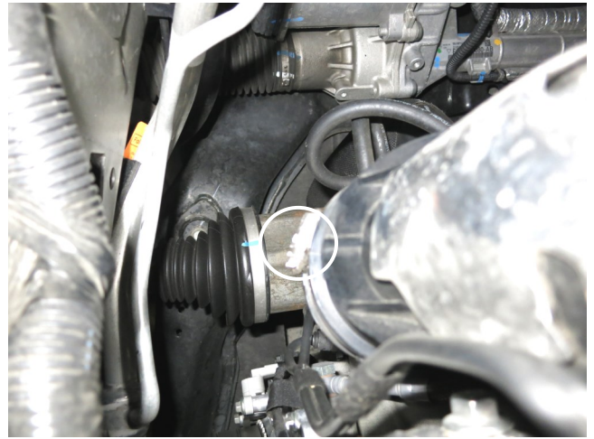
h. Loosen the hose clamp on the end of the upper intake tube.
