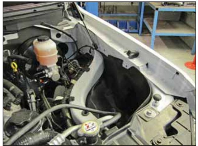
n. Remove the air box and the overflow tank assembly. NOTE: Drain the overflow tank's coolant into a clean container.
