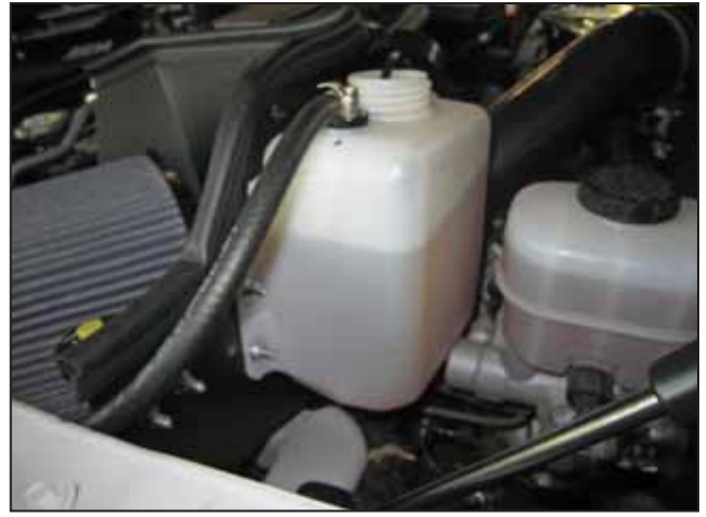
ae. Fill the AEM® overflow tank with the coolant drained from the stock overflow tank.
