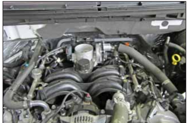
j. Intake plenum and PCV hose removed from vehicle.
