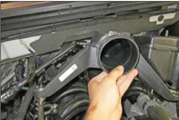
i. Remove the intake plenum along with the attached PCV hose.
