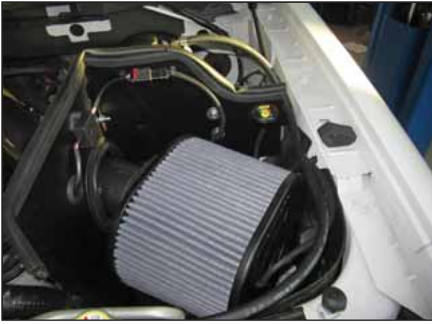
ad. Route the overflow hose to the AEM® overflow tank and install the hose clamp.
