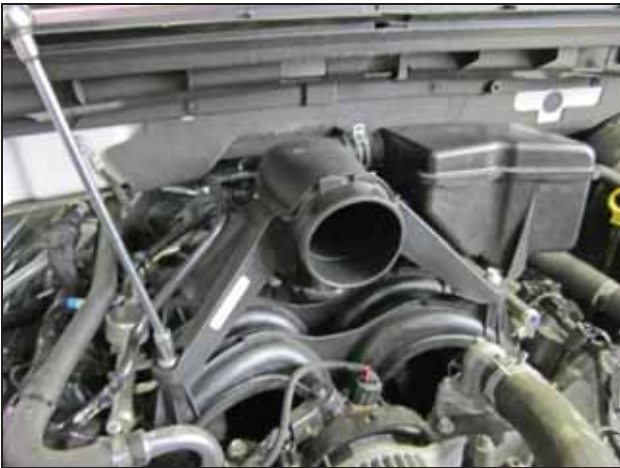
g. Remove the 4 bolts securing the intake plenum to the intake manifold.
