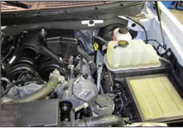
e. Remove the air box lid/inlet tube assembly.
