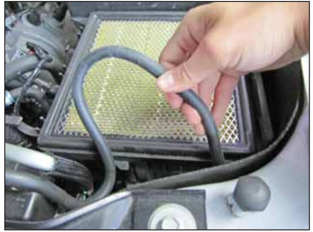
l. Pull the overflow hose out as shown.
