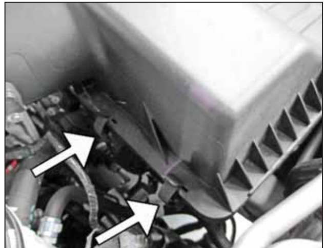
d. Unclip the 2 clips securing the air box lid to the lower air box.
