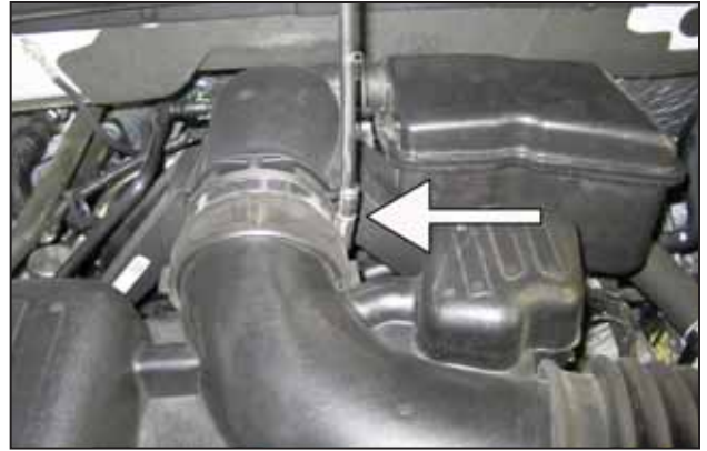
b. Loosen the hose clamp connecting the inlet tube to the intake plenum.
