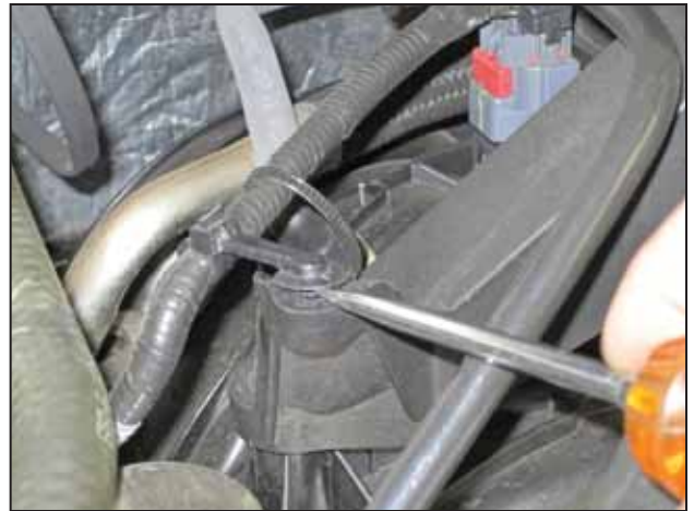
h. Unclip the zip tie secured to the rear corner of the intake plenum near the fire wall.
