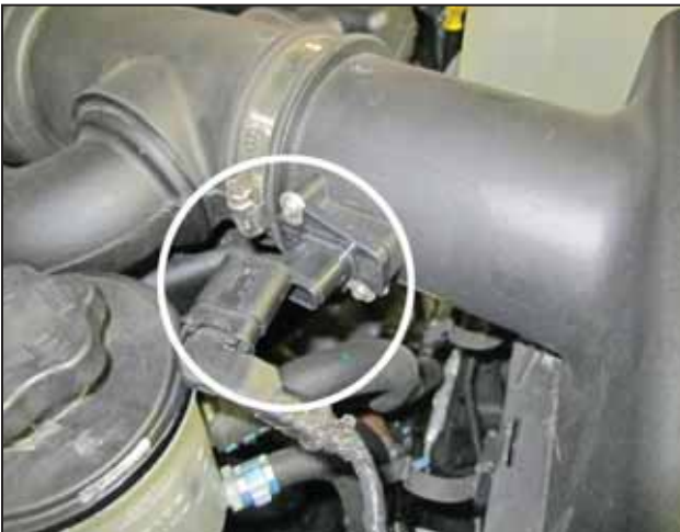
c. Disconnect the mass air flow sensor.
