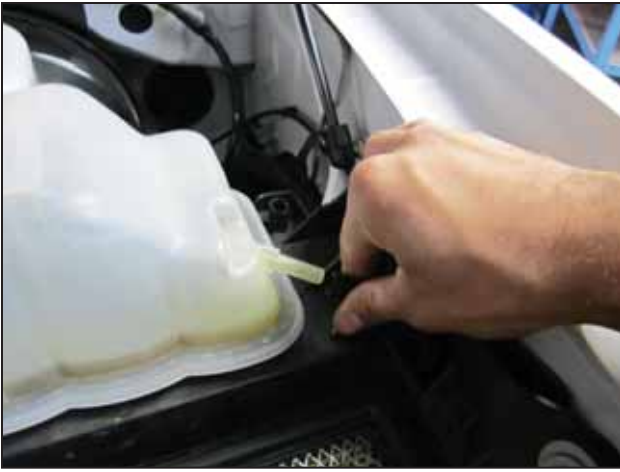
k. Disconnect the overflow hose from the overflow tank.
