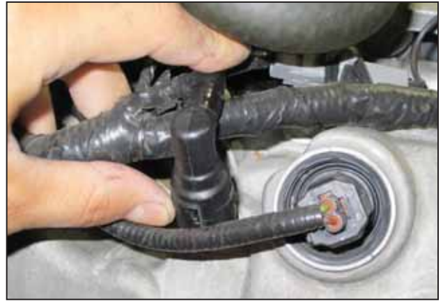
f. Disconnect the PCV hose connected to the valve cover.
