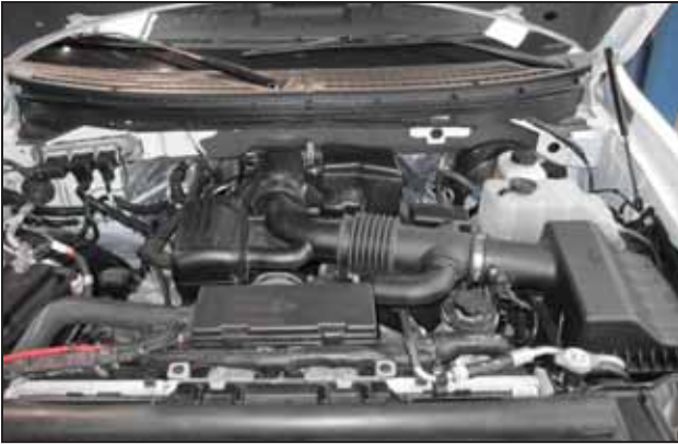
a. Stock air box system installed.
