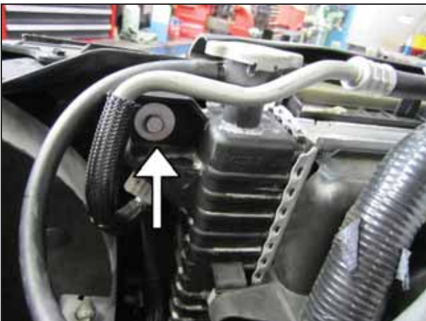
o. Remove the radiator bolt from the radiator support.
