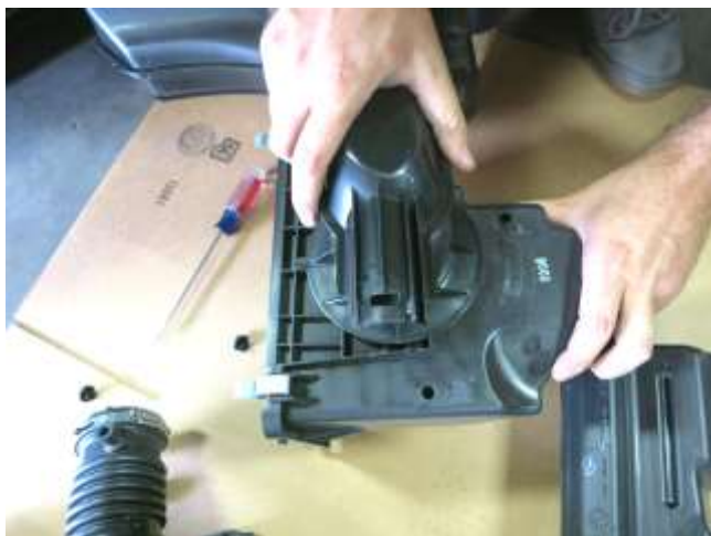
c. Rotate the cold air scoop until it will separate from the lower air box.
