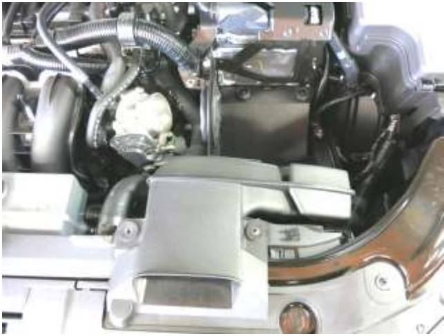
f. Insert the factory cold air scoop into the AEM heat shield and install assembly using factory grommets.
