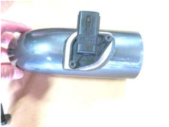
h. Install MAF sensor into the AEM intake tube using provided hardware.
