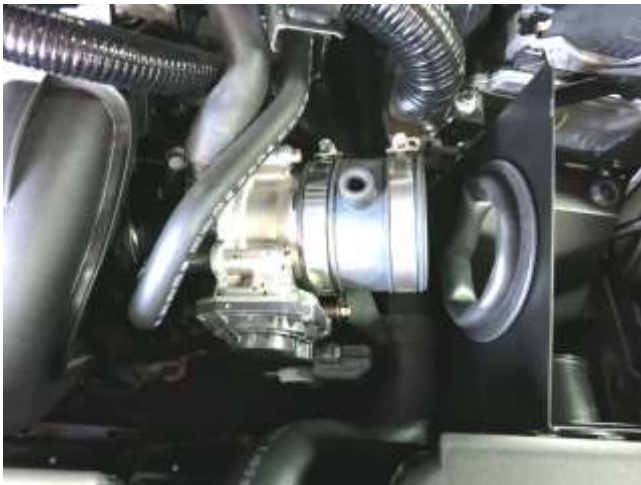
i. Install provided coupler with hose clamps provided onto throttle body with molded port facing upward. Do not tighten hose clamps at this point.
