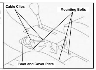
3. Enlarge the cable hole in the floor with a hacksaw or sheet metal cutters as shown in Figure #3. The enlarged portion should be at least 1" forward of the existing hole. Pull the cable boot up over the lower portion of the metal fitting on the cable. Replace the cable boot plate and leave it loose.
