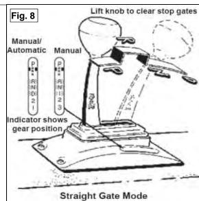
**Park:** To get to park from any straight gate position, lift the handle all the way up and push forward. The transmission will find its own Park position. Release the handle and the shifter is locked in Park. To get any other gear position, you must raise the shifter handle to clear the stop gate.
