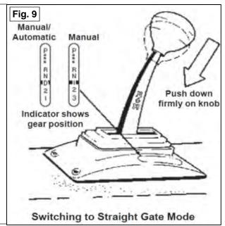
**10. Shifting and the ratchet mode:** Move the shift handle forward or backward with a quick firm action until it hits the internal stop.
