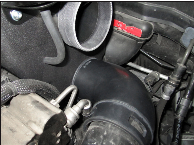
t. Insert the round end of the elbow coupler (5-1058) into the lower inlet hole of the air box. Make sure it is fully seated.
