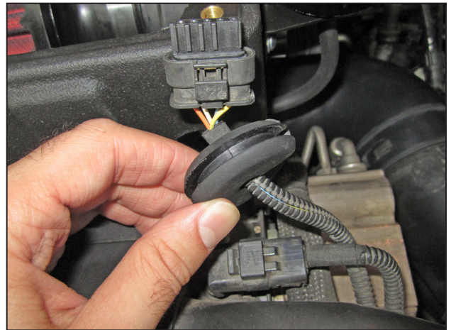
u. Place the large split grommet (784634) over the MAF wiring harness as shown. Note that that MAF harness has been re-routed underneath the other engine sensor harness to maximize slack.
