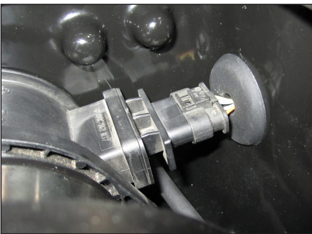
v. Connect the MAF harness connector to the MAF sensor housing inside the air box as shown.
