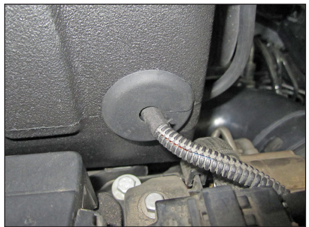
w. Fully seat the split grommet (784634) into the MAF sensor access hole in the front of the air box to completely seal the hole as shown.
