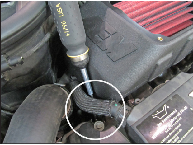
r. Align the torx screw in the mounting foot to the lower passenger side mounting pad on the intake manifold. Fully tighten the screw with a T20 Torx driver until it is fully seated in the intake manifold's mount.
