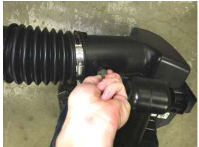
h. Remove the IAT sensor from the factory airbox by pushing and twisting counter-clockwise.
