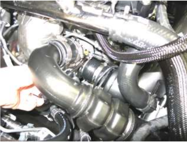
e. Lower intake tube into vehicle starting with the turbo mount end and install onto the turbo.
