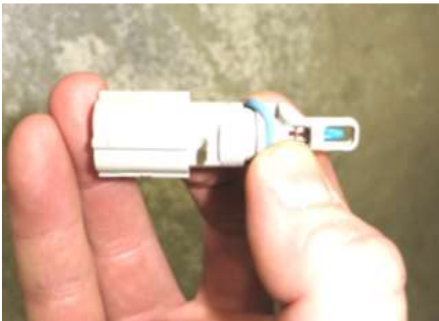
i. Carefully remove the o-ring from the IAT sensor and keep with the factory airbox.
