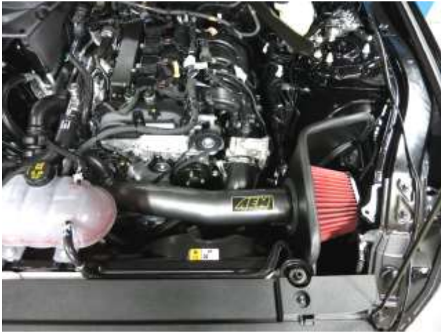
Finished installation of AEM Intake System.
