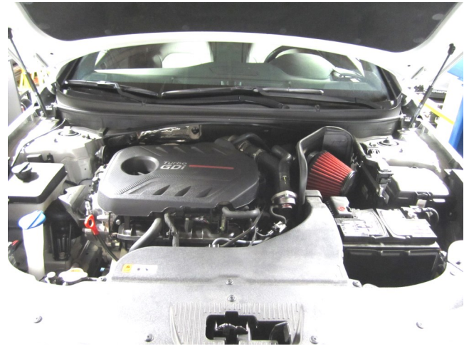
AEM Intake Installed
