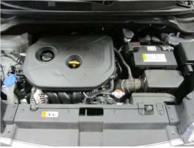
STOCK INTAKE INSTALLED
