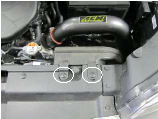
j. Re-install the engine cover and the two plastic clips holding the stock scoop in place.
