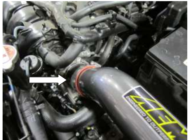
d. Install the AEM intake tube into the hose at the throttle body.
