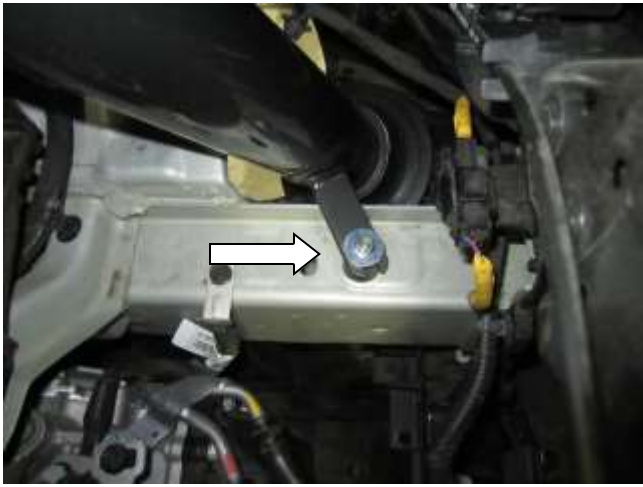
f. After the filter is installed, make sure tube alignment and filter clearance are good before tightening the two hose clamps at the throttle body. Then, tighten the nut securing the bracket to the rubber mount.
