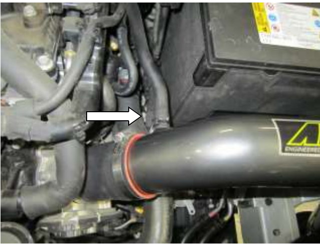
g. Connect the engine breather hose onto the AEM intake tube and secure with the pressure clamp that was removed in step 2b.
