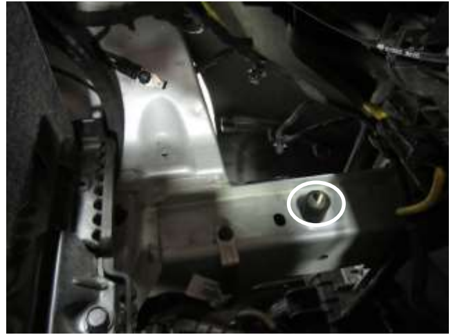
b. Install the rubber mount (1228599) onto the vehicle in the location shown.
