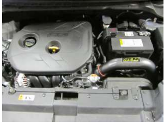
AEM INTAKE INSTALLED
