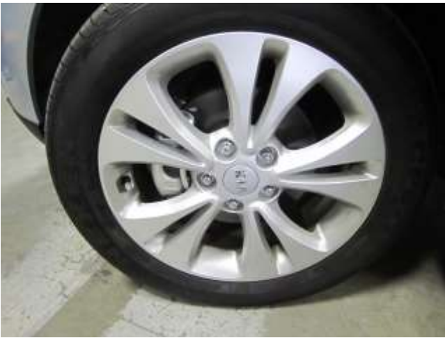
i. Re-install the drivers side wheel and torque lug nuts to manufacture specifications.
