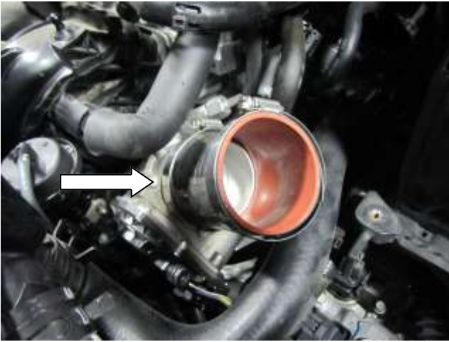
a. Install the supplied hose (5-277) and hose clamps (9444) onto the throttle body. The hose is angled, so make sure that the hose is angled up.
