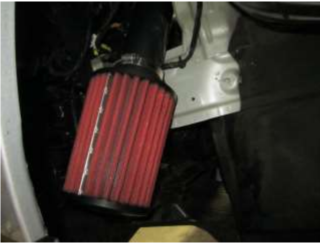
e. Install the AEM filter (21-2027DK) and hose clamp (9448) onto the AEM intake tube through the wheel well and tighten the hose clamp at this time.
