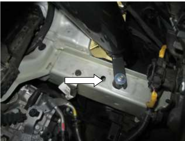
c. Install the AEM intake tube into the inner fender aligning the bracket with the rubber mount and install the washer (08160) and nut (444.460.04).
