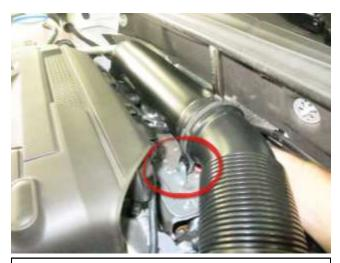
d. Remove the bolt behind the engine securing the factory intake hose to the engine.
