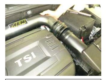
c. Slide the other coupler & clamps onto the air box end of the tube & lower the tube into position. Slide the coupler into place over the air box.
