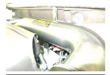
d. Reinstall the tube mounting bolt taking care to position your new intake tube with clearance all around.
