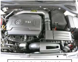
g. Finished installation of AEM Intake System.
