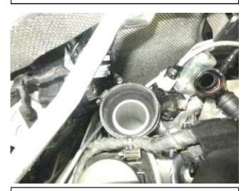
a. Install the turbo-end coupler and both corresponding hose clamps onto the turbo.
