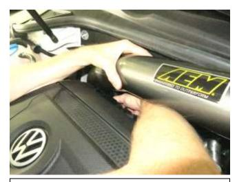
b. Rotate the end of the PCV hose & push it straight in to the port on the bottom of your new intake tube, then install the tube into the turbo-end coupler. Do not tighten clamps yet.
