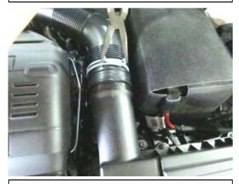
c. Disengage the spring clamp retaining the factory intake hose to the air box and disconnect the tube from the air box.
