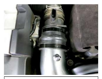
g. Install the supplied coupler, clamps, and intake tube onto the factory MAF sensor and align the tube bracket to the rubber mounted stud.
