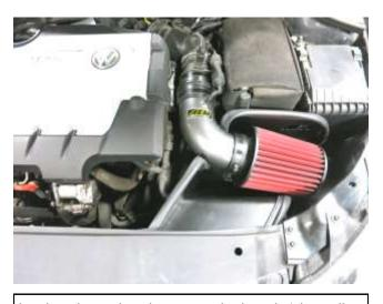
I. When the intake tube is properly aligned, tighten all hose clamps and tighten the M6 nut securing the intake tube bracket.
