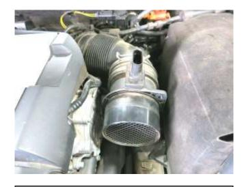
d. Install the MAF sensor into the factory turbo inlet hose. Note: Pay attention to the air flow direction, the screen side of MAF sensor should face the front of the vehicle.
