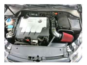
n. AEM air intake system installed
