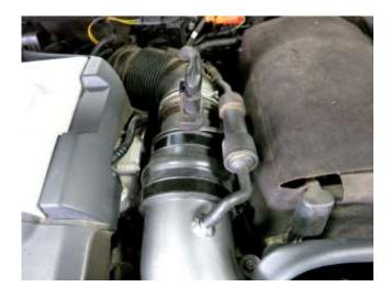
$\ensuremath{k}.$  Connect the vacuum line to the fitting on the AEM intake tube.
