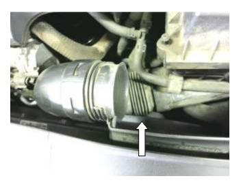
f. Disconnect the air duct from the lower air box and remove from vehicle. **Note: Removing the duct allows** for easier air box removal.
