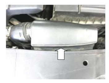
c. Unclip and remove the fresh air scoop from the air inlet and separate it from the lower air duct to the air box.
