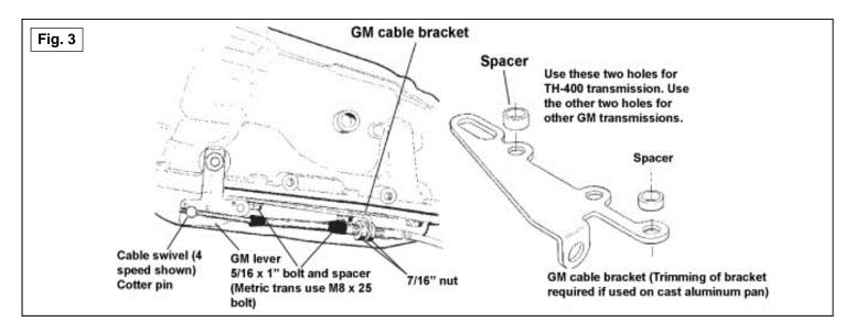
11. Move the transmission selector lever by hand to full rear position (Low). Operate the shifter lever to the Low gear position (ratcheted all the way back). Adjust the large nuts on the cable so that the swivel will slide into the center hole on the selector lever. Tighten the large nuts completely. Be sure that the swivel will slide freely in and out of the hole in the selector lever.
