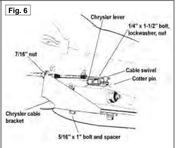
20. Remove the two transmission oil pan bolts directly below the shift lever. Install the cable bracket in position (See Fig. 6) with two spacers between the pan and the bracket. (If your transmission is equipped with a cast aluminum oil pan these spacers can be omitted.) Install the two 5/16-18 x 1.00" pan bolts supplied and tighten to 12-13ft.lbs. Do not overtighten as this can damage the pan gasket.
