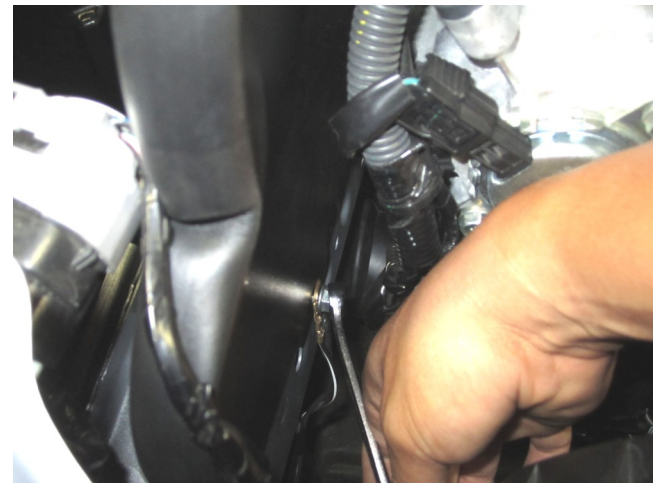
d. Install the M6 bolt from 2i) onto the lower heat shield along with the ground wire back as shown.
