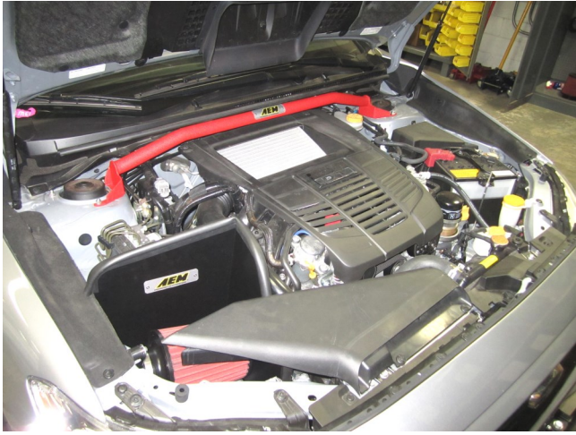
n. AEM intake installed.
