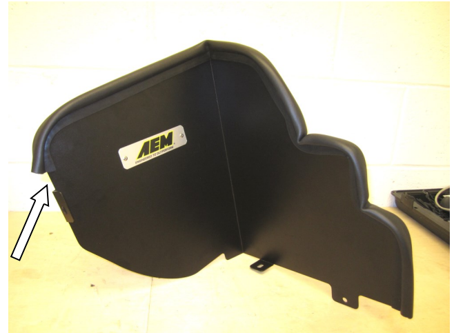
b. Install the supplied edge trim(102496) onto the outer part of the heat shield leaving a 1 inch gap near the left mounting tab. Cut excess edge trim if necessary.
