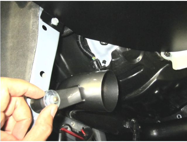
k. Use supplied nut(444.460.04) and washer(08160) to secure upper tube bracket to rubber mount.
