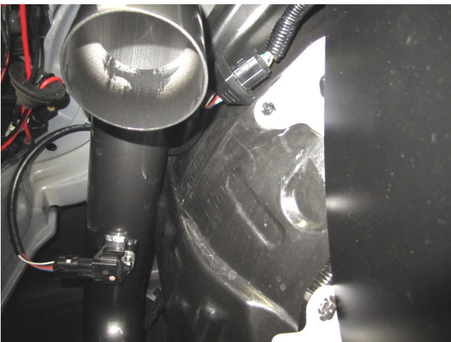
i. Connect the MAF extension harness(8-197-1) to the stock harness, around the tube, and plug into the MAF sensor.
