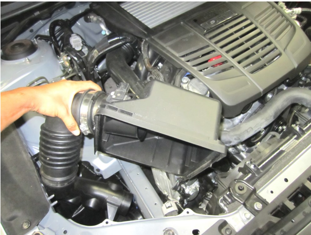
g. Slide the intake tube off the lower bellow coupler and remove tube/box assembly from engine bay.
