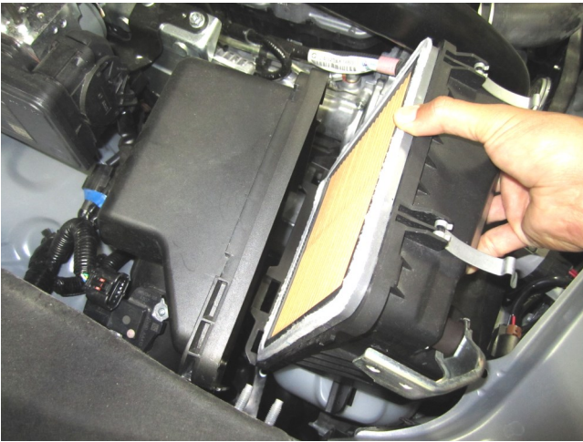
e. Unlatch and carefully remove the stock air box lid and filter from the engine bay.
