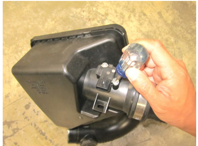
h. Remove MAF sensor from stock air box and set aside for installation on AEM intake tube.
