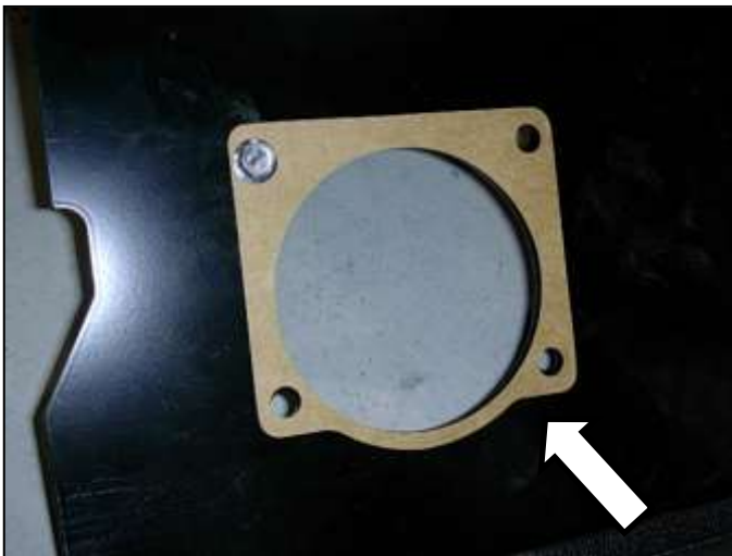
f. Place one of the supplied gaskets onto each side of the large hole in the heat shield.
