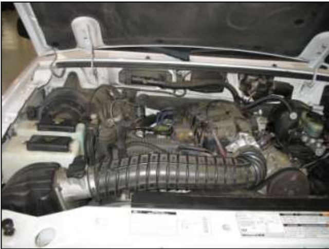
a. Factory air box system installed.
