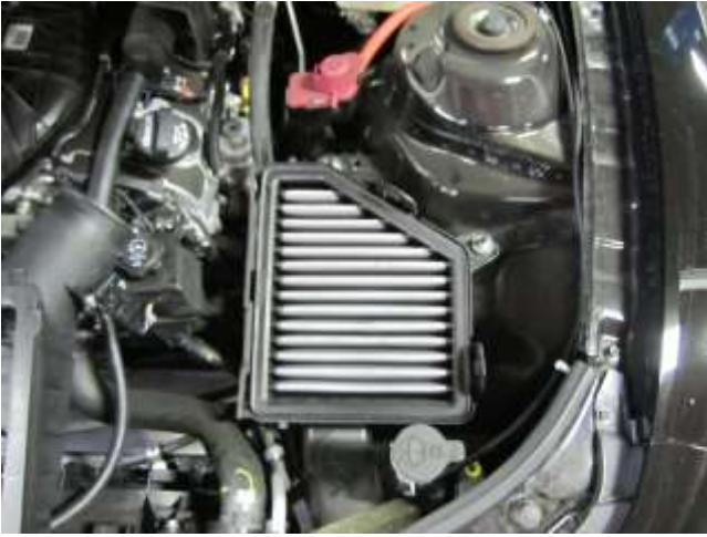
a. Install the AEM air filter into the air box base as shown.
