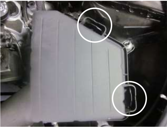
e. Unclip the two tabs retaining the air box lid and remove the lid to expose the stock air filter.
