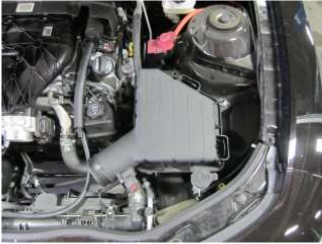
b. Install the air box lid back onto the air box base making sure the tabs latch.
