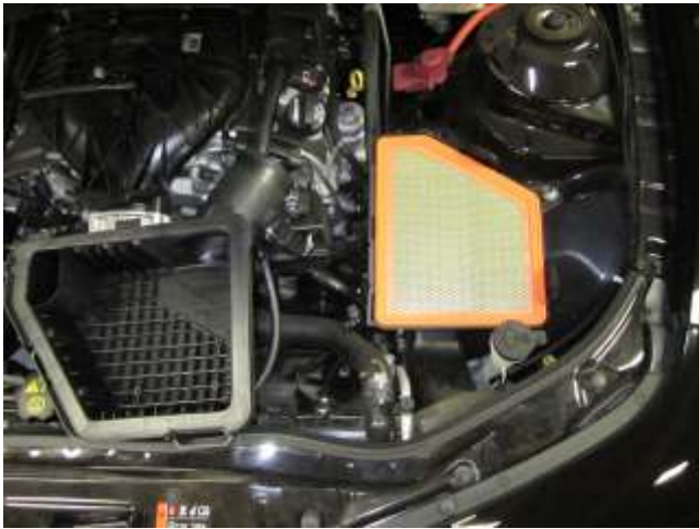
f. Remove the stock filter from the lower air box.
