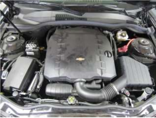
Factory air box system installed
