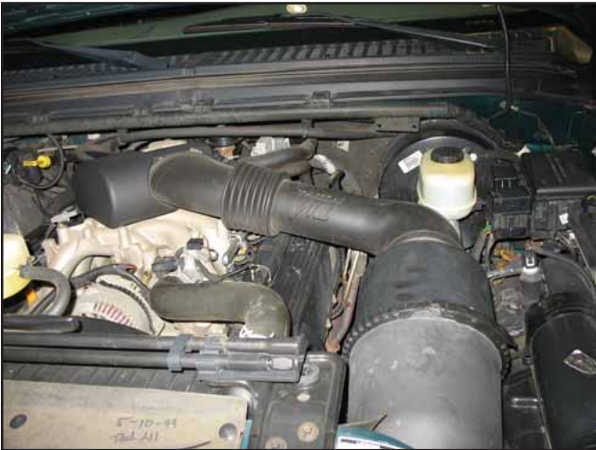
a. Factory air box system installed.
