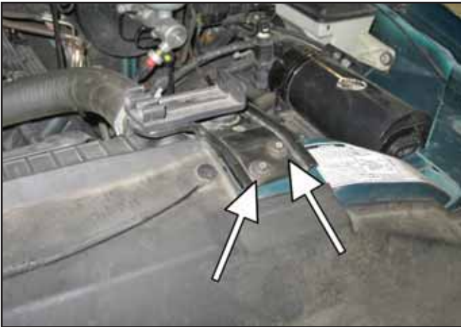
c. Remove the two bolts securing the radiator support bracket located on the driver side of the engine bay. Remove the radiator support bracket.
