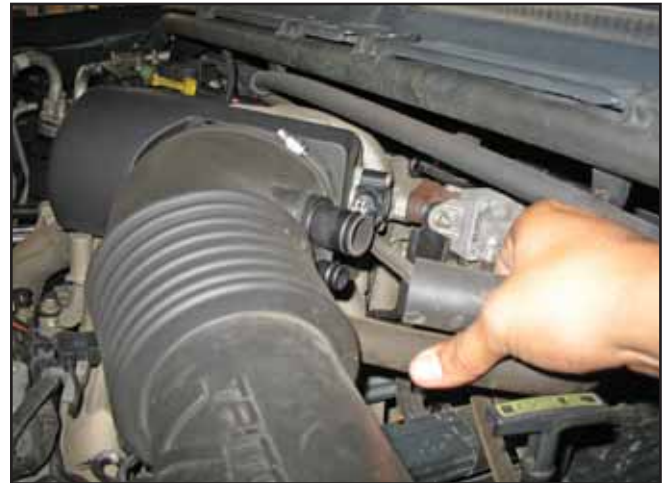
d. Remove the two stock breather hoses from the upper intake tube. Loosen the hose clamp securing the upper intake tube to the throttle body.
