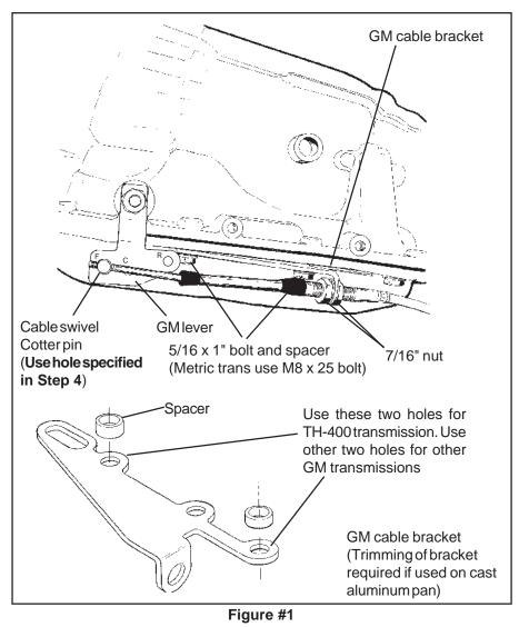
might be required for the 4L80E and 4L85E. Verify that selector lever does not grind on cable bracket before moving on to step 3.
