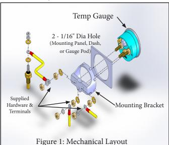
Rotate gauge until it is properly aligned and tighten each nut finger tight.
