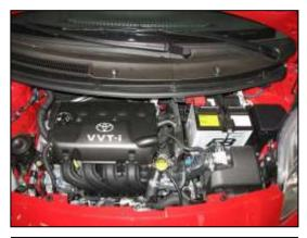
a. Factory airbox system installed.
