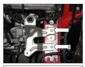
i. Remove the two bolts securing the airbox mounting bracket. Release the wire harness clip from the underside of the airbox mounting bracket. Remove the airbox mounting bracket from the engine bay.
