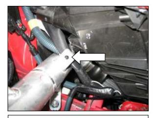
m. If the wire harness behind the headlight rubs the intake pipe, secure it to the mounting tab with one of the supplied pushmount zip ties. Ensure the wire harness is NOT in tension. Depending on the length of the wiring harness, this step may not be necessary.
