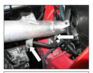
n. Route the MAF sensor connector wire harness under the intake pipe as shown. Secure the harness in two places using the remaining two push-mount zip ties.
