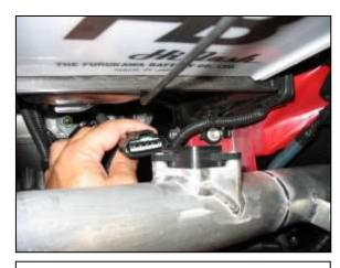
I. Plug in the MAF sensor connector to the MAF sensor.
