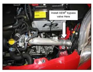
If you choose to install an AEM® bypass valve (sold separately) install it in the location specified. Refer to the AEM® bypass valve installation instructions to ensure proper installation.
