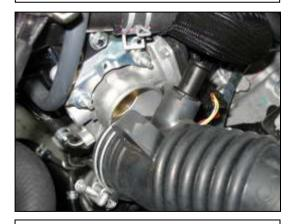
e. Loosen the hose clamp and pull the intake tube clear of the throttle body.
