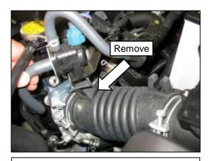
c. Pull the EVAP VSV mounting clip free from the intake tube. Remove the Phillips head screw that secures the mounting bracket to the EVAP VSV.
