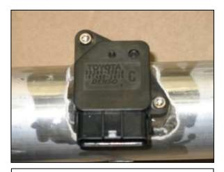
d. Install the MAF sensor into the AEM<sup>®</sup> intake pipe. Secure with the two provided 8-32 socket bolts. Use care during the installation to avoid damaging the o-ring.
