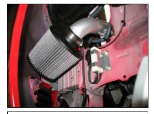
k. Install the AEM® air filter onto the end of the intake pipe. Slide it on until the shoulder inside the air filter is flush with the end of the pipe. Secure with the supplied 2.15-3.00" hose clamp.
