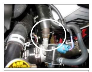
h. Attach the crankcase breather hose to the intake pipe and secure in place with the factory spring clamp.
