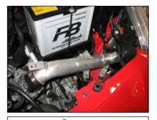
e. Install the AEM® intake pipe into the engine bay. Align the mounting bracket onto the rubber mount installed in step 3b. Insert the other end of the intake pipe into the coupler installed on the throttle body.
