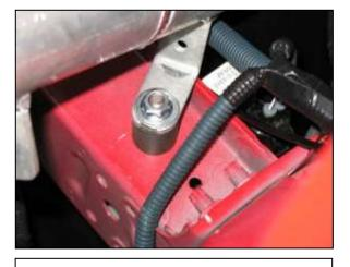
f. Loosely secure the pipe's mounting bracket to the rubber mount with the supplied M8 washer and nut.
