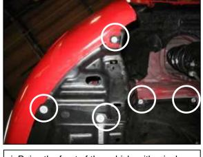
i. Raise the front of the vehicle with a jack. Refer to your owner's manual for proper jack and jack stand placement to properly support vehicle. Support your vehicle using properly rated jack stands before wheel removal or while working under the vehicle. NEVER WORK UNDER A VEHICLE WITHOUT USING JACK STANDS. Remove the driver side wheel. Remove the five screws securing the lower splash quards.
