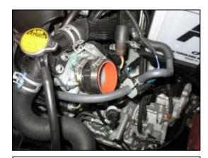
c. Install the silicone coupler onto the throttle body. Loosely install the two 2.25" hose clamps.
