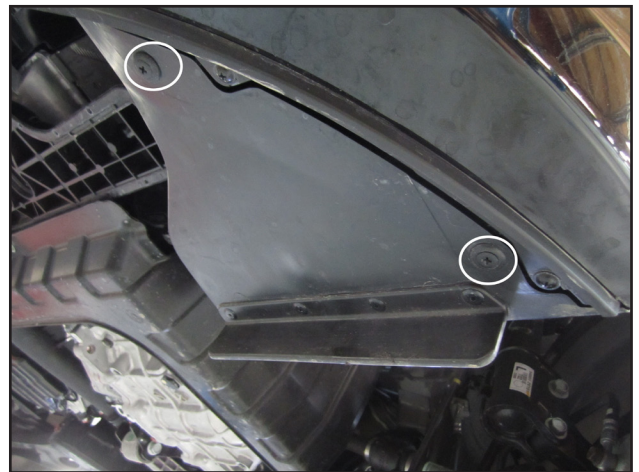
h. Remove the two plastic clips under vehicle, near driver's side front wheel to lower plastic wheel well liner.
