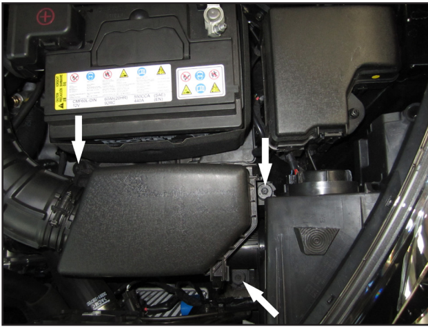
e. Remove the three M6 bolts securing the stock airbox
