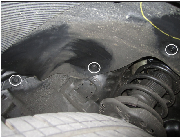
g. With the vehicle raised, remove the three plastic clips in the driver side front wheel well as indicated above.
