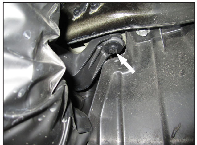
j. From driver's side wheel well, remove the M6 bolt used to secure the intake resonator chamber rear mount.
