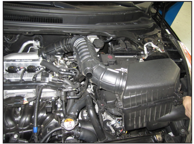
f. Firmly grasp the airbox and slide it towards the engine to detach from lower chamber. Remove stock intake airbox and tube assembly.
