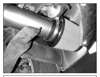
k. Install the air filter on the end of the intake pipe. Ensure the splash guard is properly installed and allows clearance for the intake pipe.
