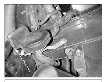
j. Rotate the horn bracket forward out of the way of the intake pipe.
