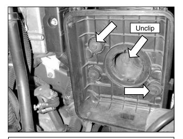
d. Remove the three bolts holding the other half of the air filter box. Unclip the box from the air inlet tube and remove the assembly from the engine bay.
