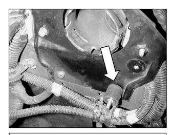
c. Install the rubber mount in the hole exposed from step 3b.
