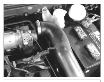
b. Disconnect the intake tube from the throttle body.
