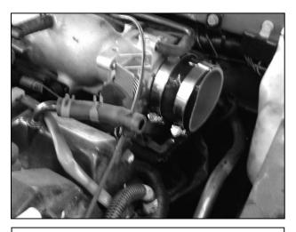
d. Install the silicone coupler on the throttle body. Place the hose clamps in place but do not tighten them.
