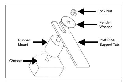
Proper installation of rubber mount assembly
