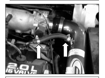
g. Insert the intake pipe into the engine bay. Place the end of the intake pipe into the silicone coupler on the throttle body. Do not tighten the hose clamps. Install the 3/8" hose and hose clamps from the PCV tube to the nipple on the intake pipe as shown.
