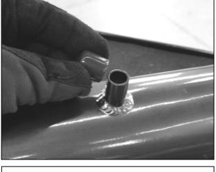
e. Some non-California vehicles are equipped with an air injection hose leading from the exhaust to the stock inlet pipe. This hose must be re-connected to the AEM® inlet pipe. If your vehicle is not equipped with this hose use the 5/8" cap to plug the fitting on the AEM® inlet pipe.
