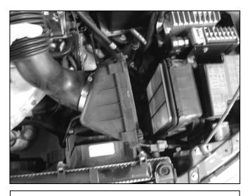
c. Unclip the air filter box and remove the intake tube from the engine bay. Remove the air filter.
