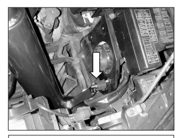
i. Line up the bracket on the intake pipe with the rubber mount. Install the nut and washer according to the diagram below. After proper fitment has been achieved, tighten the hose clamps on the throttle body and tighten the nut on the rubber mount.
