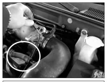
a. Loosen the hose clamp on the throttle body and disconnect the PCV hose from the intake tube.
