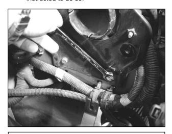
b. Remove the lower front bolt from the air box backing plate as shown in the picture.
