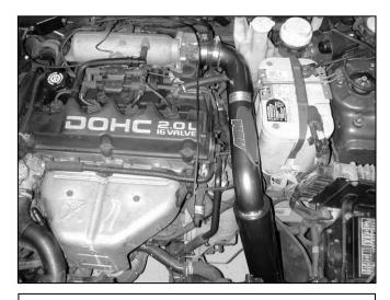
h. Position the intake pipe in the engine bay so that no part of it touches the vehicle.
