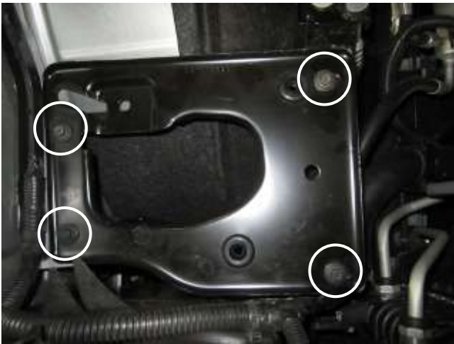
e. Loosen and remove the four M6 bolts. Then, remove the air box plate from the vehicle. These will not be re-used. Note: Do not discard the plate or hardware.
