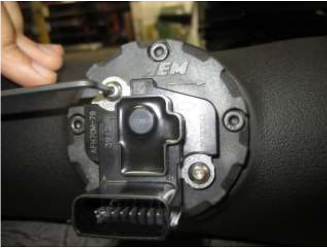
c. Install the mass air sensor into the mass air sensor adapter that has already been attached to the AEM intake tube with the provided M4 allen's. Note: Be very careful with the mass air sensor.
