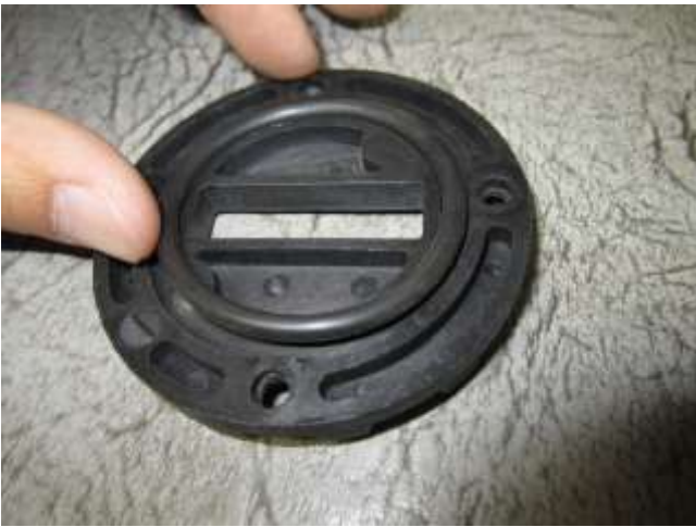
a. Install the provided O-ring into the mass air sensor adapter.
