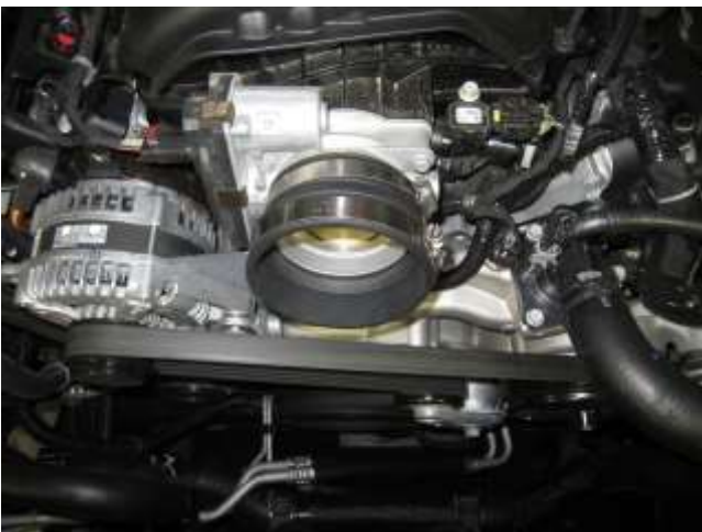
g. g. Install the throttle body coupler with hose clamps 5.3L use p/n 341018 and #56; 6.2L use p/n 341014 and #64. Do not tighten clamps at this point.
