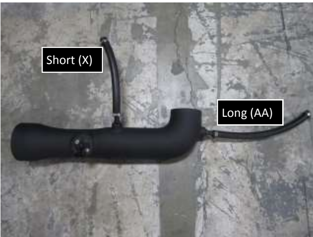
e. Slide the two supplied vent hoses and four clamps onto the vent fittings and tighten. The shorter hose will go on the left vent, and the longer hose will go on the right vent.
